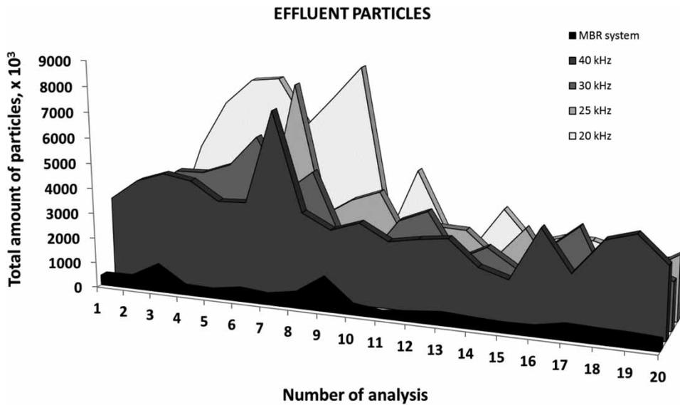
Figure 4 | Presence of particles in the effluent of the conventional MBR system and sonicated modules at different sonication frequencies.
