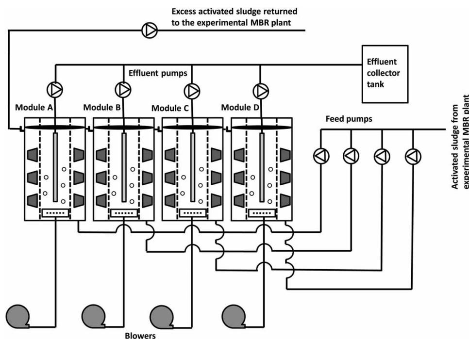
Figure 1 | Schematic experimental setup.
