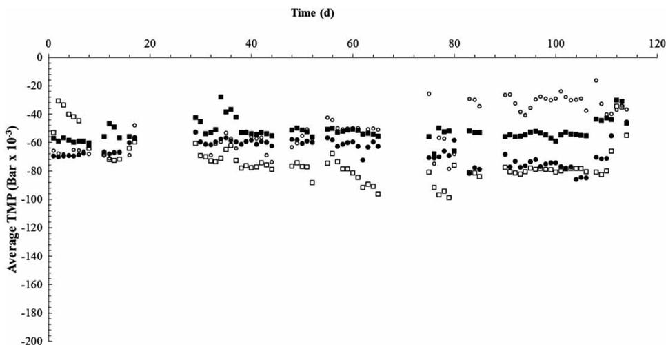
Figure 2 | Time course of average daily TMP in sonicated modules at 20 (○), 25 (●), 30 (□) and 40 (■) kHz of sonication frequencies.
