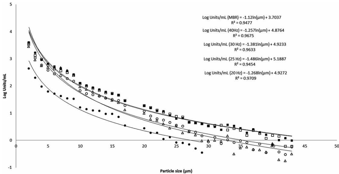
**Figure 5** | PSD (2–125  $\mu\text{m}$ ) for effluent from conventional MBR (●), and Ultrasound MBR at 40 Hz (□), 30 Hz (○), 25 Hz (Δ) and 20 Hz (■).
