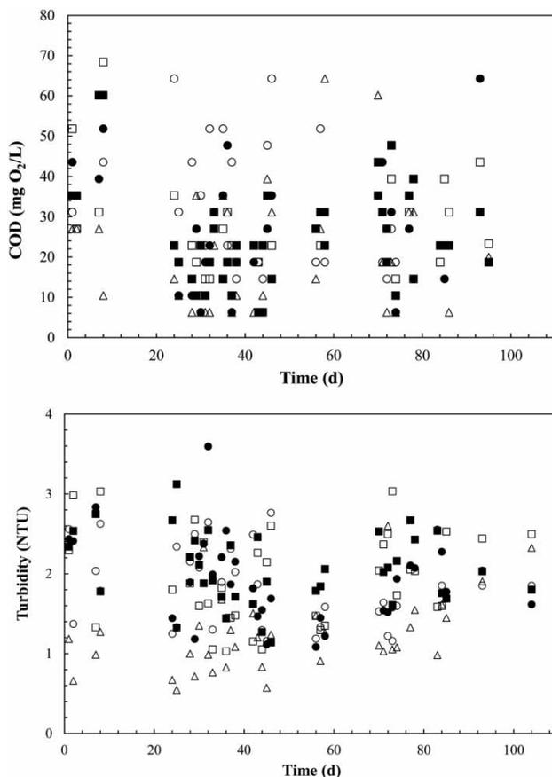
**Figure 3** | Effluent COD concentration and turbidity in the conventional MBR system ( $\Delta$ ) and in sonicated modules at 20 (O), 25 (●), 30 (□), and 40 (■) kHz of sonication frequencies.
