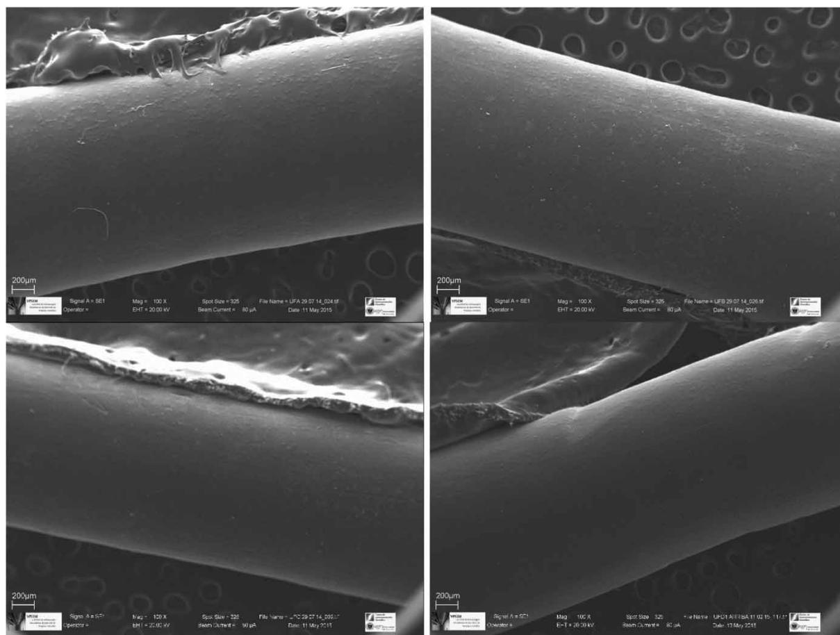
**Figure 6** | SEM images of the membrane surfaces after sonication at 40 kHz (top left), 30 kHz (top right), 25 kHz (bottom left) and 20 kHz (bottom right).
