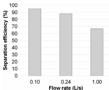
Figure 2 | Separation efficiencies of the lamella system at different flow rates according to the DIBt test method.
