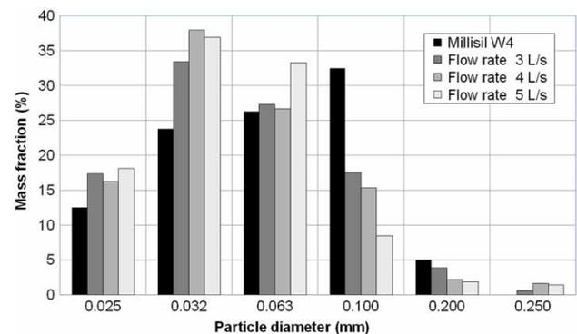
**Figure 4** | Mass fractions of different size ranges of Millisil W4 washed out from the manhole of the lamella system at high hydraulic loadings.
