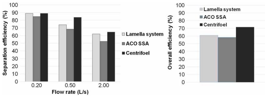
**Figure 3** | Separation efficiencies of the lamella system and of two commercial systems at different flow rates according to the HS-OWL test method.
