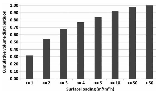
**Figure 7** | Cumulative volume distribution of water flow rates through the system derived from 1 min average values as a function of surface loading.
