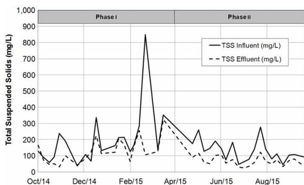
**Figure 5** | Influent and effluent TSS concentrations of the lamella system during the field study.
