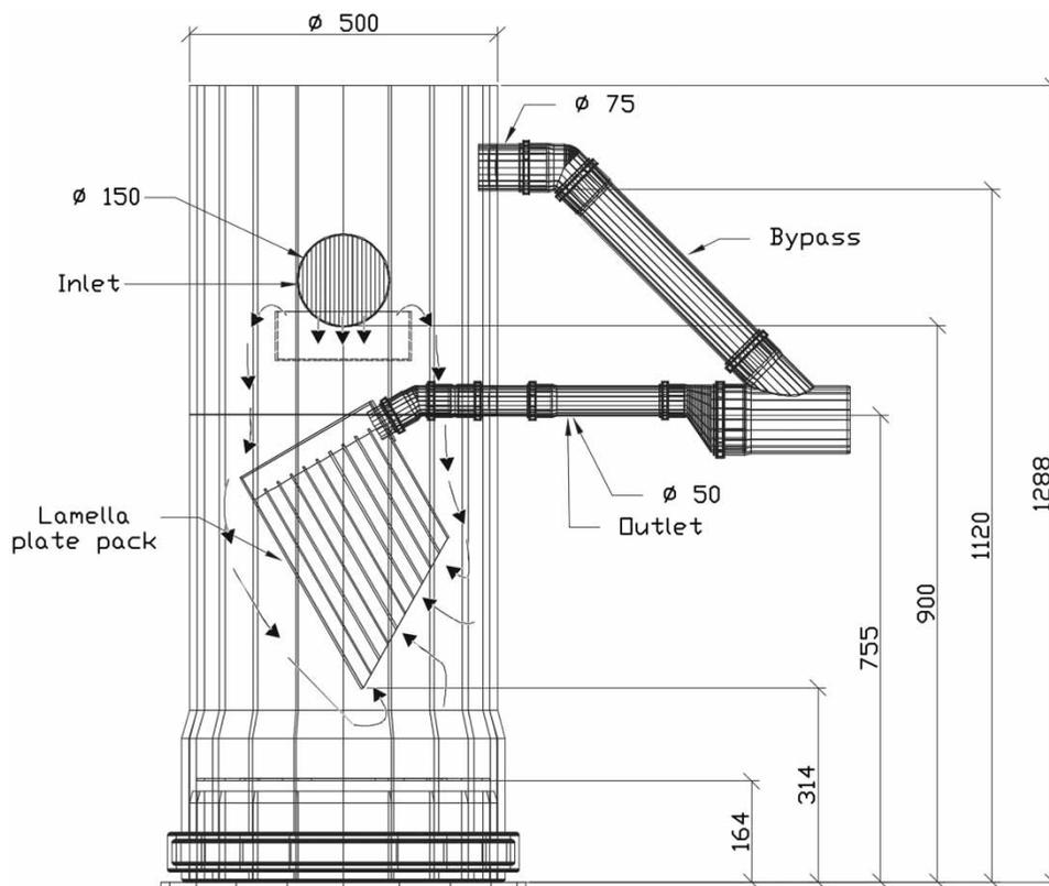
Figure 1 | Decentralised lamella plate settler developed in this study (unit: mm).
