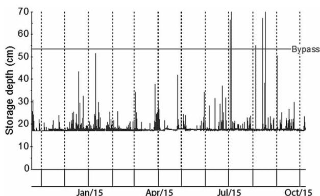
**Figure 6** | Time series of the recorded storage depths in the decentralised system during the field study.
