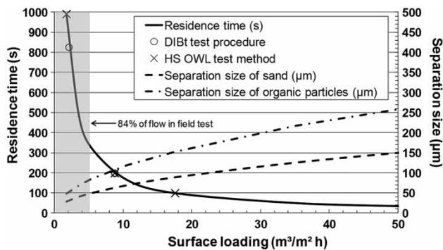
**Figure 8** | Residence time and separation size of two different materials as a function of surface loading of the lamella system (filling volume = 198 L).
