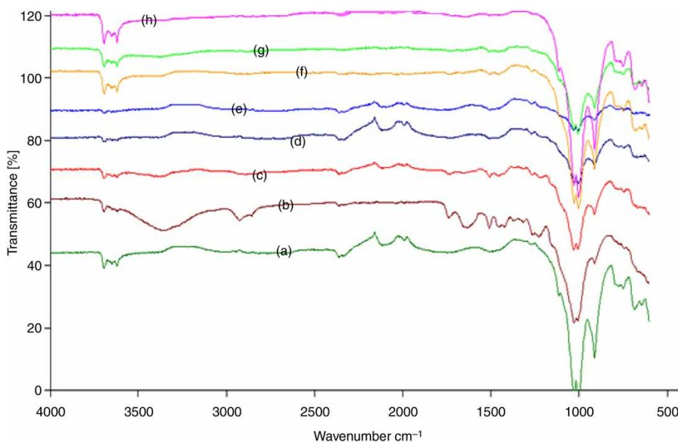
**Figure 1** | FTIR spectra for (a) MMT:SD:PH (9:0.5:0.5), (b) MMT:SD:PH (8:2:2), (c) MMT:SD:PH (7:1.5:1.5), (d) MMT:SD:PH (6:2:2), (e) MMT:SD:PH (5:2.5:2.5), (f) MMT:SD:PH (4:3:3), (g) MMT:SD:PH (3:3.5:3.5), (h) MMT:SD:PH (2:4:4).
