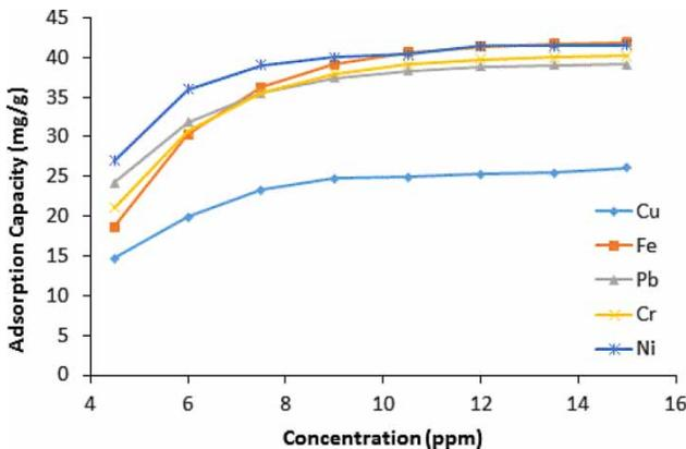
**Figure 9** | Effect of initial heavy metal ion concentration on adsorption for ternary composite.
