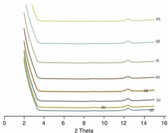
**Figure 2** | XRD scan for (a) MMT:SD:PH (9:0.5:0.5), (b) MMT:SD:PH (8:2:2), (c) MMT:SD:PH (7:1.5:1.5), (d) MMT:SD:PH (6:2:2), (e) MMT:SD:PH (5:2.5:2.5), (f) MMT:SD:PH (4:3:3), (g) MMT:SD:PH (3:3.5:3.5), (h) MMT:SD:PH (2:4:4), (i) MMT:SD:PH (1:4.5:4.5), (h) MMT:SD:PH (2:4:4).
