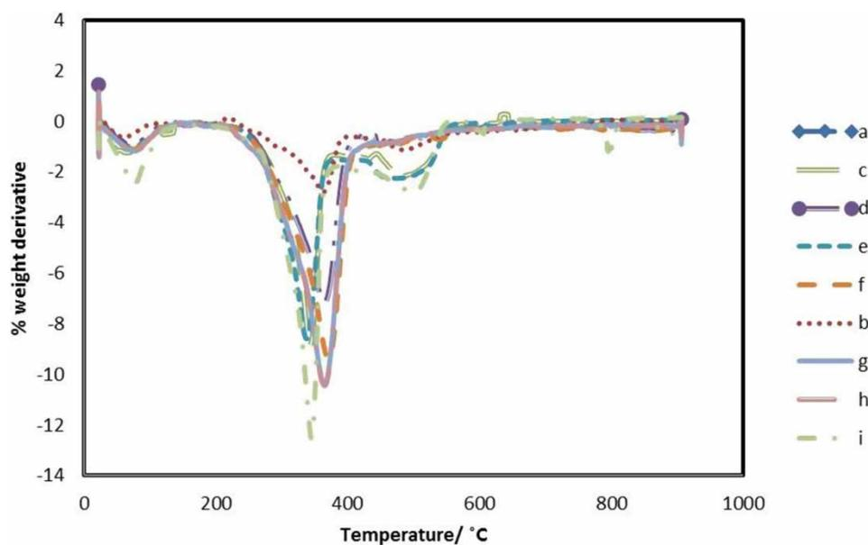
**Figure 3** | DTG curve for (a) MMT:SD:PH (9:0.5:0.5), (b) MMT:SD:PH (8:1:1), (c) MMT:SD:PH (7:1.5:1.5), (d) MMT:SD:PH (6:2:2), (e) MMT:SD:PH (5:2.5:2.5), (f) MMT:SD:PH (4:3:3), (g) MMT:SD:PH (3:3.5:3.5), (h) MMT:SD:PH (2:4:4), (i) MMT:SD:PH (1:4.5:4.5).
