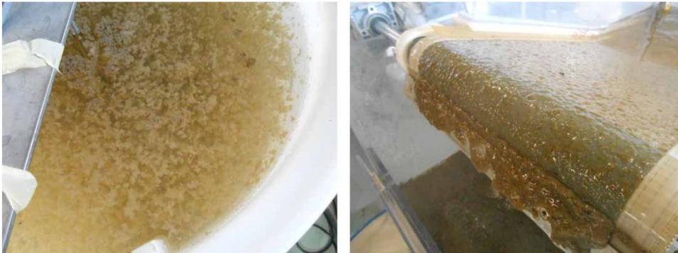
**Figure 9** | Flocs from pilot-scale flocculation of MBBR effluent with PAX-18 and polymer (left), and scraper removing flocculated biofilm solids from the early prototype RBS belt (right).
