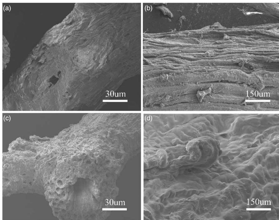
Figure 2 | The SEM image of (a), (b) LF and (c), (d) LF-AA.
