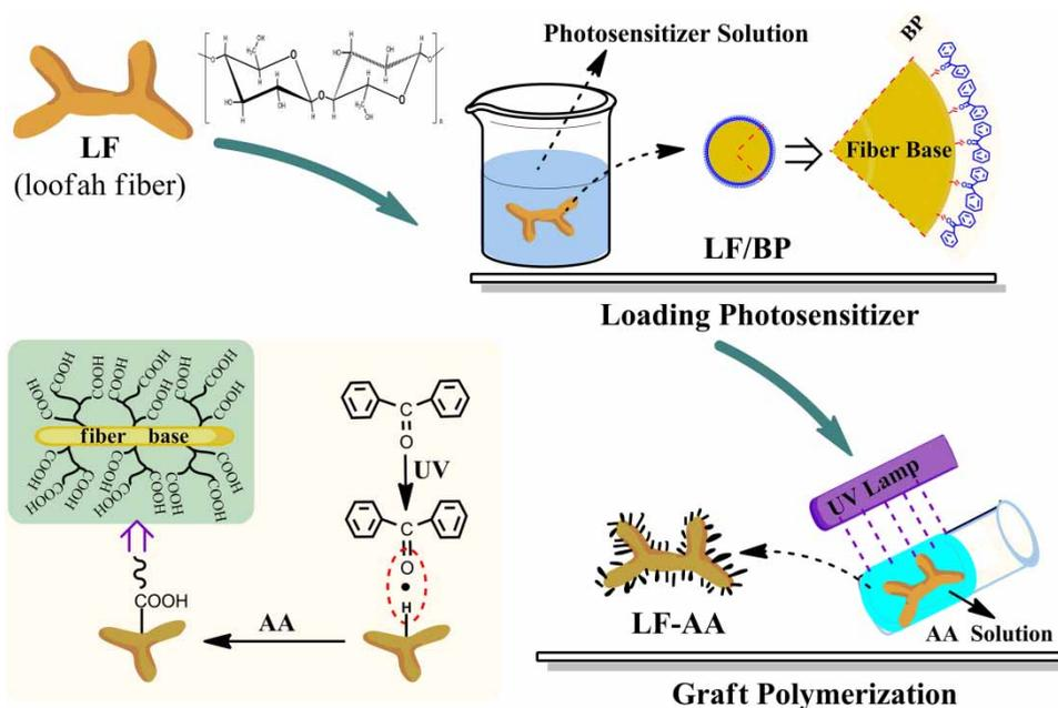
Figure 1 | Scheme of preparation of LF-AA composite.
