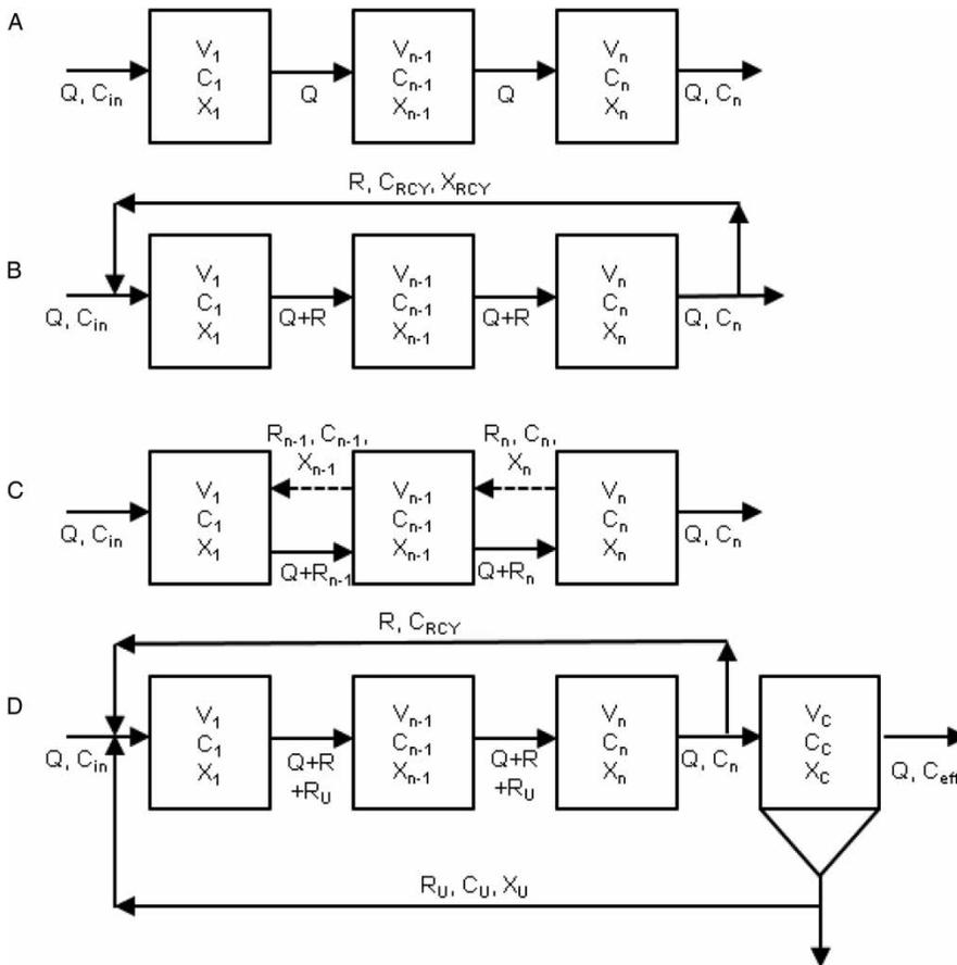
**Figure 1** | Biofilm reactor hydrodynamic models: *Configuration A* with  $X_{\text{carrier}}$  constrained in each CFSTR, *Configuration B* with  $X_{\text{carrier}}$  migration through a series of  $n$  CFSTRs, *Configuration C* with  $X_{\text{carrier}}$  migration and back-mixing, and *Configuration D* with  $X_{\text{carrier}}$  migration throughout an MLE process and coupled liquid-solid separation unit.
