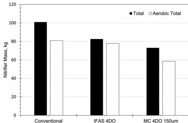
**Figure 7** | Comparison of simulated autotrophic nitrifier mass in the entire system (left) with that in the aerobic CFSTRs (right). IFAS – integrated fixed-film activated sludge; DO – dissolved oxygen; MC – mobile [biofilm] carrier.
