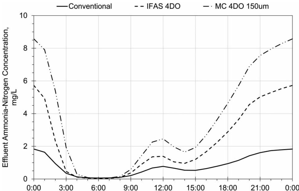
Figure 6 | Diurnal profile of the bulk-liquid ammonia-nitrogen concentration for the suspended growth system ( $S_{B,O_2} = 2 \text{ g/m}^3$ ), the IFAS system ( $S_{B,O_2} = 4 \text{ g/m}^3$ ), and the migrating  $X_{\text{carrier}}$  system ( $S_{B,O_2} = 4 \text{ g/m}^3$ ,  $L_F = 150 \mu\text{m}$ ).
