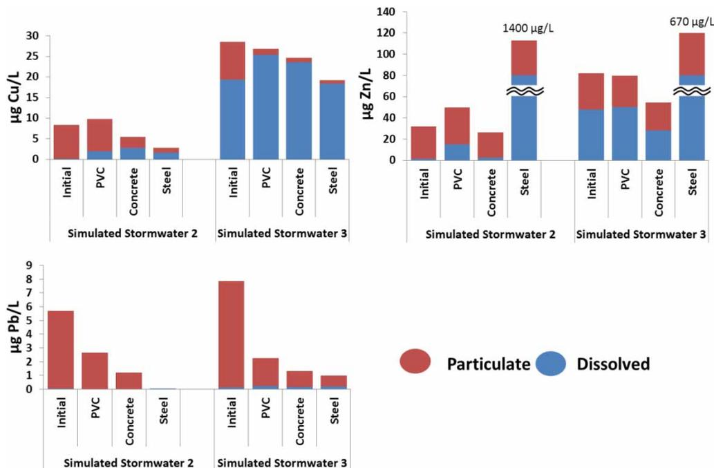
**Figure 3** | Concentrations of dissolved (blue) and particulate (red) metals in stormwaters SW2 and SW3: before and after circulation in pipes made of concrete, galvanized corrugated steel, and PVC. Please refer to the online version of this paper to see this figure in colour: <http://dx.doi.org/10.2166/wst.2017.195>
