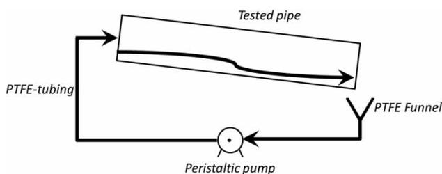
Figure 1 | Sketch of the experimental apparatus.
