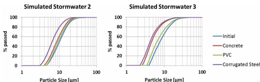
Figure 2 | PSDs by numbers of particles in simulated stormwaters SW2 and SW3 before (initial) and after circulation through the test apparatus.
