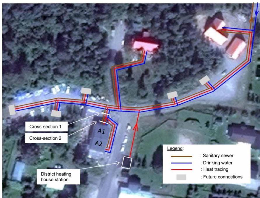
**Figure 1** | Aerial view over the pilot site. The district heating pipes are not visualised here. The full colour version of this figure is available in the online version of this paper, at <http://dx.doi.org/10.2166/wst.2017.174>.
