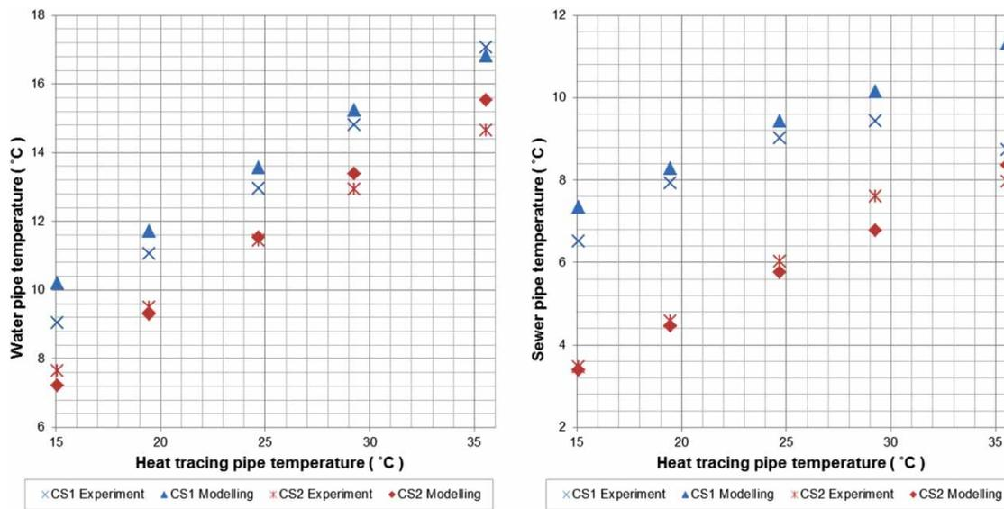
**Figure 4** | Comparison of experimental and modelling results. Influence of heat tracing temperature on water (left) and sewer temperature (right) at cross sections 1 and 2.
