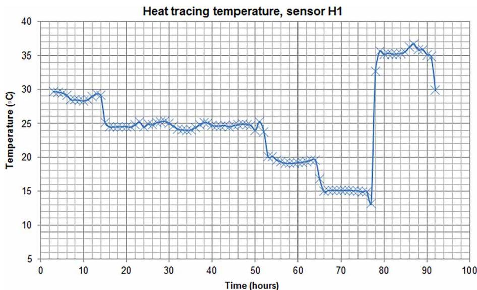
**Figure 3** | Heat tracing pipe temperature applied at cross section 1 during the experiment.
