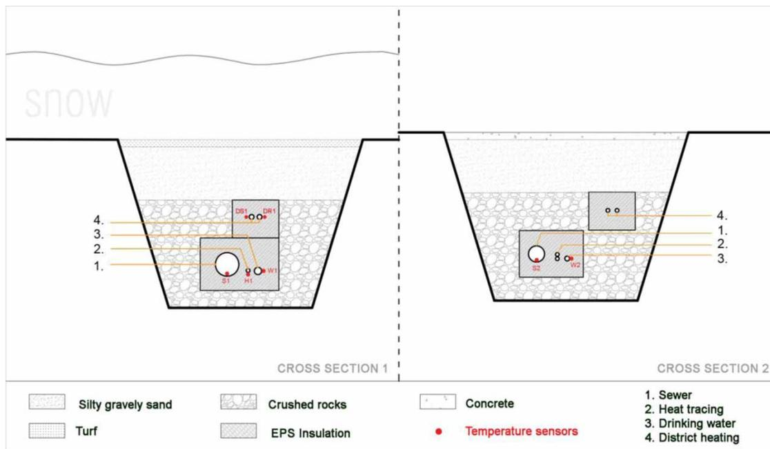
**Figure 2** | Geometries of the studied cross sections and temperature sensors' locations. The full colour version of this figure is available in the online version of this paper, at <http://dx.doi.org/10.2166/wst.2017.174>.
