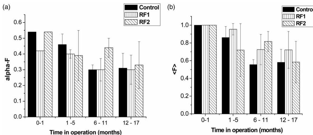
Figure 3 | Impact of reverse flexing (RF) on the evaluated weighted; (a) alpha fouling ( $\alpha F$ ) and (b) fouling factor (F) of the polyurethane Messner panel diffusers over time in operation.
