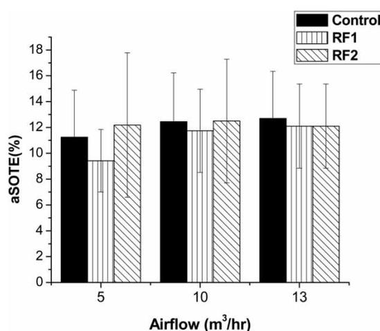
**Figure 4** | Comparing evaluated oxygen transfer efficiency ( $\alpha$ SOTE) standardized to process conditions at three different standardized airflow of 5 m<sup>3</sup>/h, 6 m<sup>3</sup>/h and 8 m<sup>3</sup>/h.
