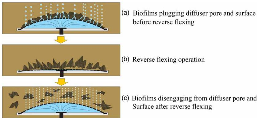
**Figure 1** | Description of the reverse flexing process and the resultant effect.
