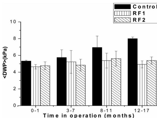
**Figure 2** | Impact of reverse flexing (RF) on weighted dynamic wet pressure (DWP) of polyurethane Messner panel diffusers over time in operation.
