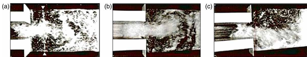
Figure 1 | Plane view of hydraulic jump in sudden diverging basin; (a) normal, (b) with negative step and (c) with central sill (Bremen (1990), reproduced with kind permission of the author).
