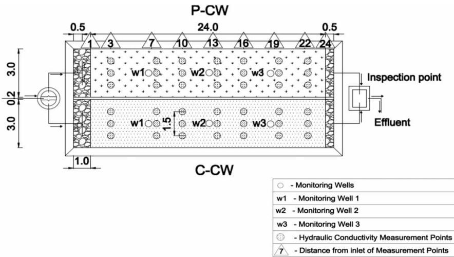
Figure 1 | Constructive details of HSSF-CW and evaluation positions of saturated hydraulic conductivity.
