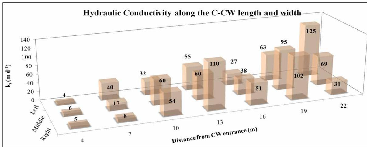
Figure 7 | Saturated hydraulic conductivity using FHM, at several points in the unplanted control wetland.
