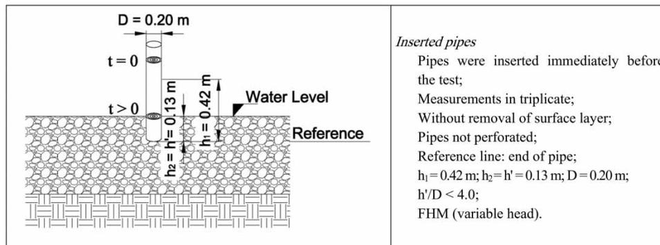
Figure 2 | Conditions for the implementation of FHM hydraulic conductivity tests on saturated medium. The pipes were inserted before testing.
