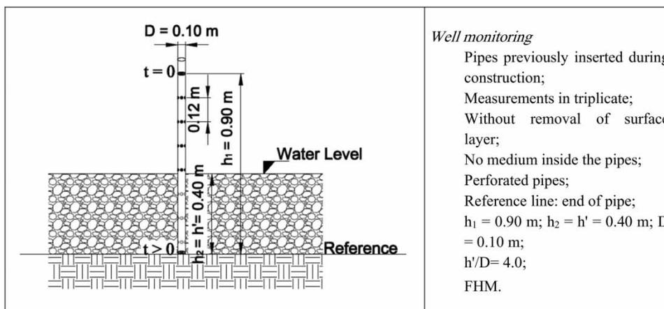
Figure 3 | Conditions for FHM hydraulic conductivity tests using the existing monitoring wells.
