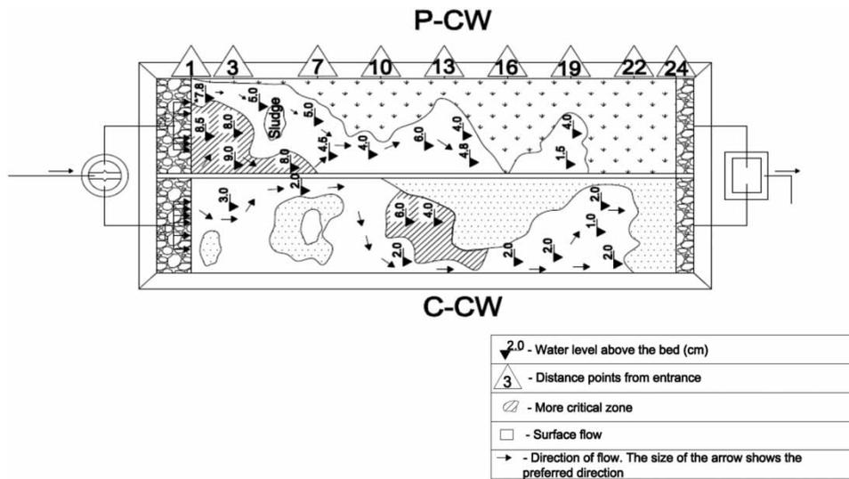
Figure 6 | Visual analysis of the wetland conditions, with indication of visible surface flow and the presence of a water level above the bed surface.
