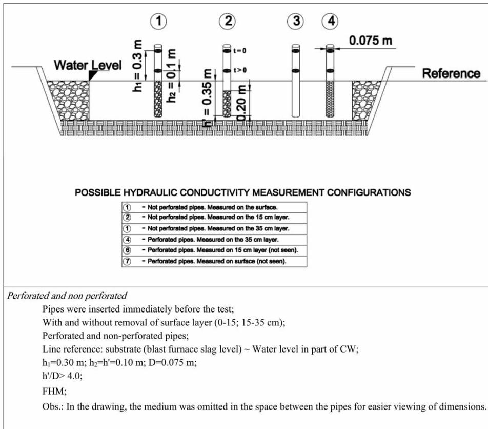
**Figure 4** | Conditions for the implementation of FHM hydraulic conductivity tests by using perforated and non-perforated pipes.
