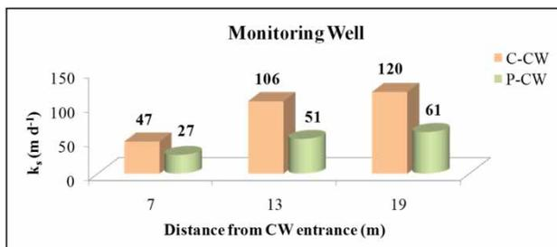
**Figure 9** | Saturated hydraulic conductivity measured in monitoring wells located at different points in the HSSF-CW.
