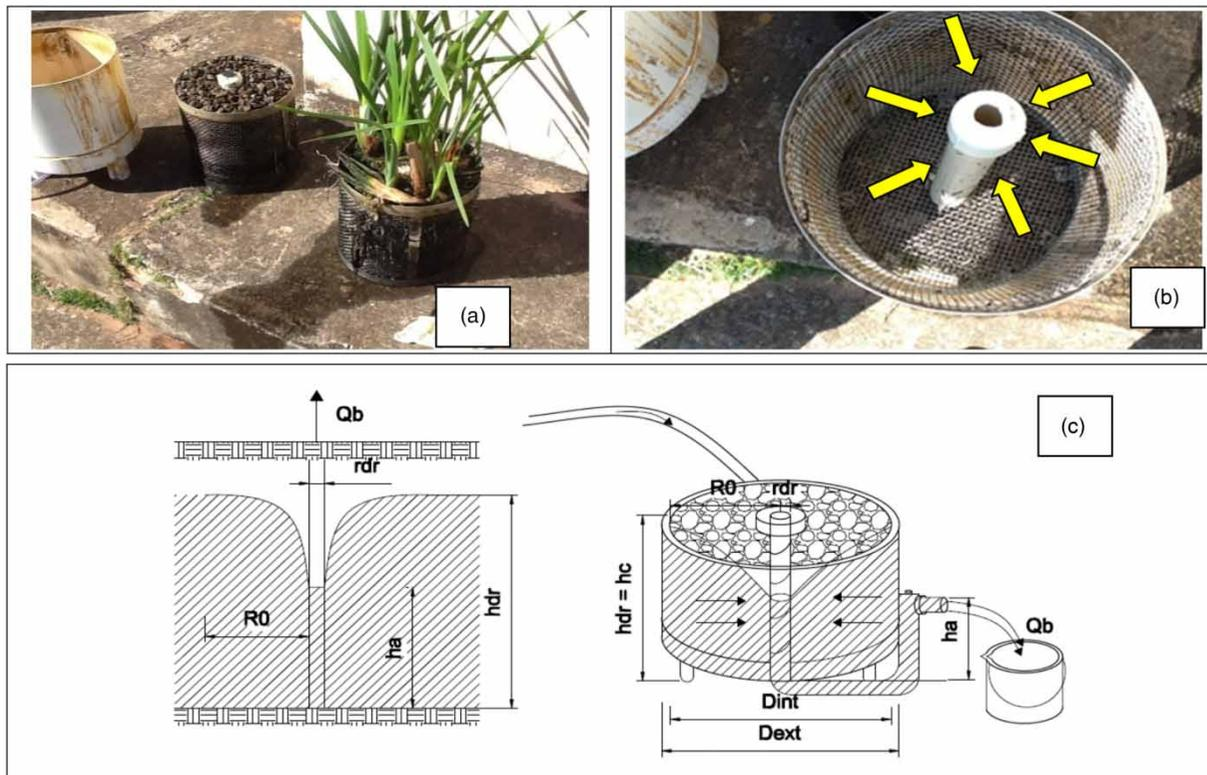
**Figure 5** | (a) Detail of PFR removed from the baskets from the unplanted and planted units; (b) the water flow direction inside the PFR baskets; (c) analogy between the hydraulic conditions in the experimental apparatus used to determine the hydraulic conductivity of saturated medium (right) and pumping wells in an unconfined aquifer (left).
