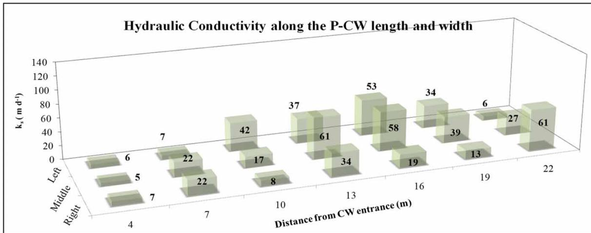
**Figure 8** | Saturated hydraulic conductivity using FHM, at several points in the planted wetland.
