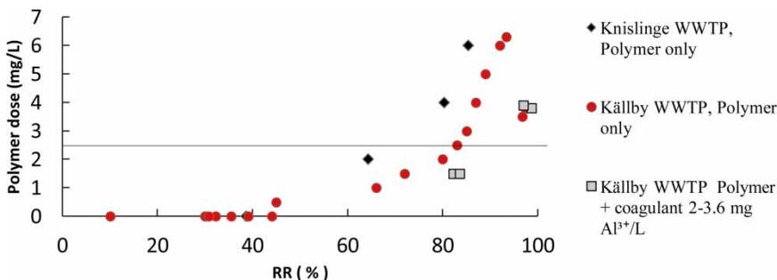
**Figure 2** | Correlation between polymer dose and required reduction (RR). Knislinge WWTP (data retrieved from Väänänen et al. (2016)), Knislinge and Källby WWTP, Sweden. Straight line shows maximum feedforward polymer dose.
