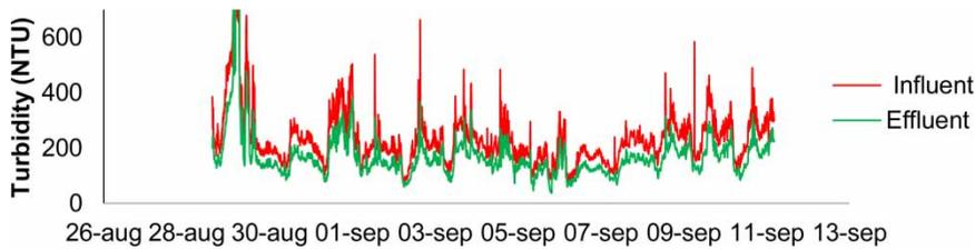
**Figure 3** | Pilot experiment results; influent and effluent turbidity from 14 days of continuous operation without chemical dosing: 100  $\mu\text{m}$  filter media,  $Q_m$  40  $\text{m}^3/\text{h}$ .
