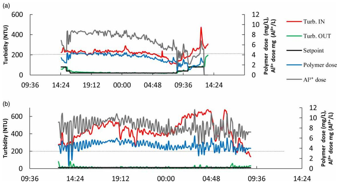
**Figure 7** | Result from set point step test, (a) 80, 40, 20, 40, 80 NTU,  $C_f=2$ ,  $40 \text{ m}^3/\text{h}$ ; and (b) 12 NTU test,  $C_f=1.8$ ,  $40 \text{ m}^3/\text{h}$ . Influent turbidities above the dotted line (200 NTU) show feedforward and feedback control simultaneously in operation and influent turbidities below the dotted line (200 NTU) show feedback control only.
