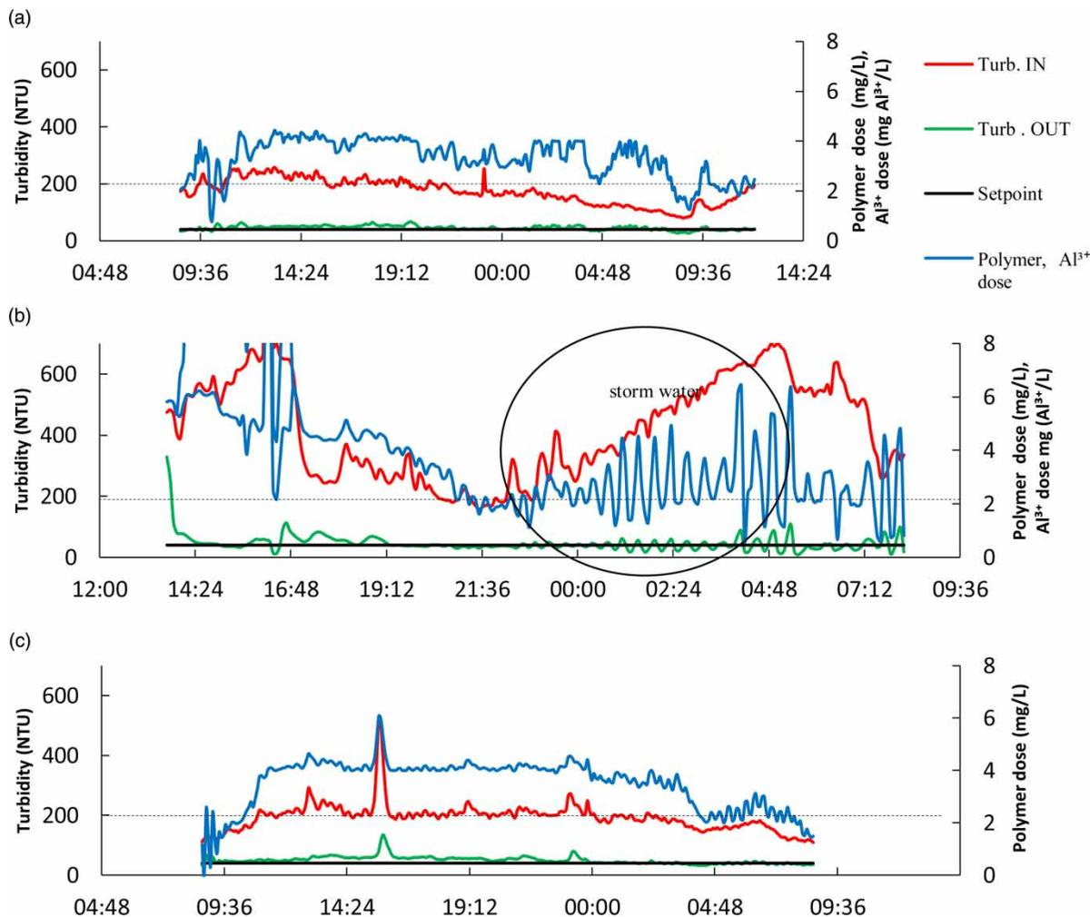
**Figure 5** | 40 NTU tests: (a) 15 m<sup>3</sup>/h,  $C_f = 1$ , (b) 40 m<sup>3</sup>/h,  $C_f = 2$  and reduced to 1 (@16:48), with storm water treatment during the night (00:00–05:00) and (c) 40 m<sup>3</sup>/h,  $C_f = 0$ . Influent turbidities above the dotted line (200 NTU) show feedforward and feedback control simultaneously in operation and influent turbidities below the dotted line (200 NTU) show feedback control only.
