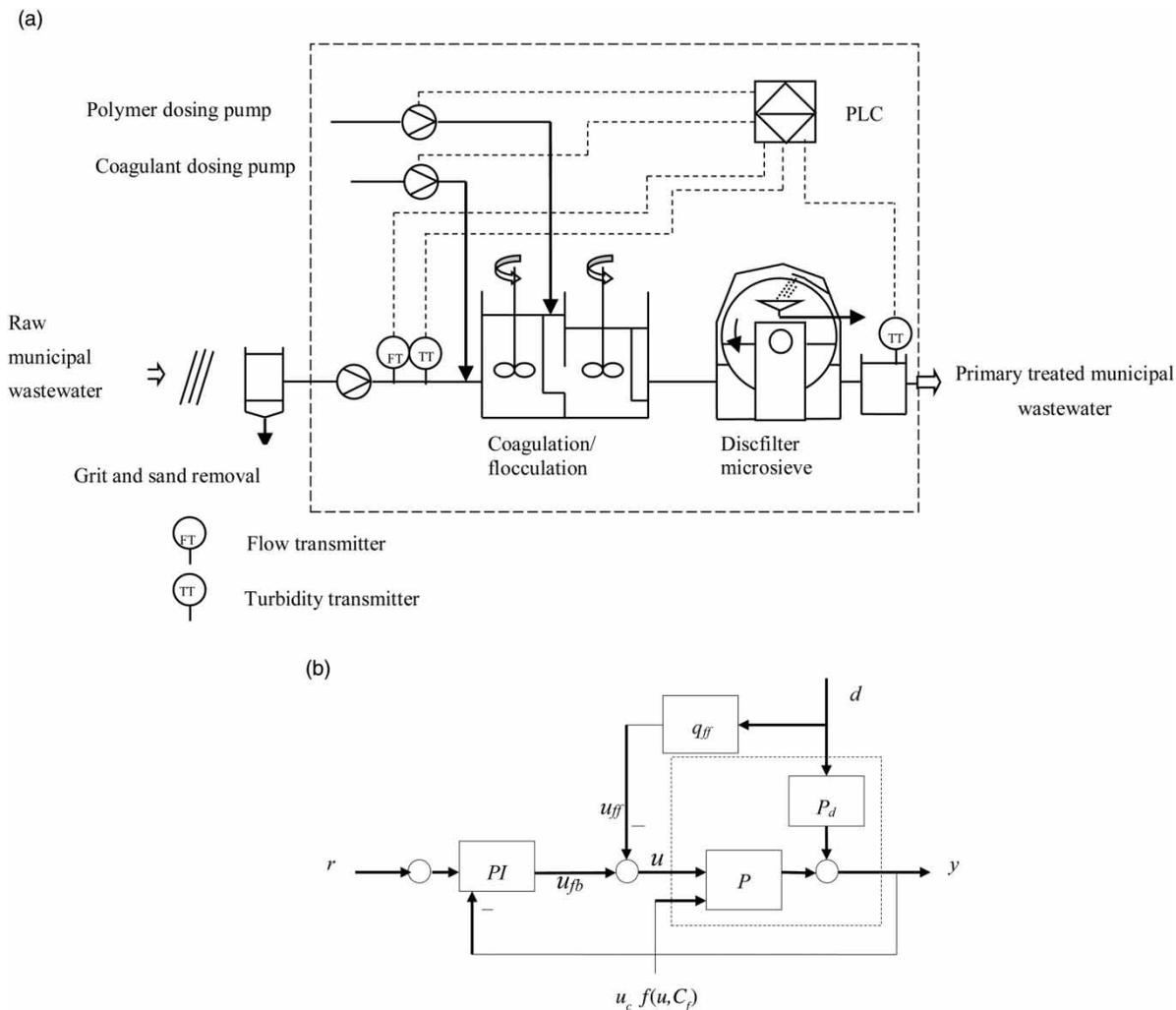
**Figure 1** | (a) Schematic illustration of the pilot plant and control system and (b) block diagram of the control structure.
