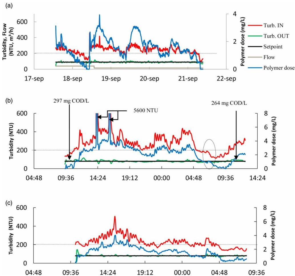
**Figure 6** | 90 NTU test: (a) stepwise decrease in flow from 40–15 m<sup>3</sup>/h. Set point experiment with 80 NTU and two flow regimes: (b) 15 m<sup>3</sup>/h,  $C_f = 0$ , effluent COD from grab samples are shown, and (c) 40 m<sup>3</sup>/h  $C_f = 0$ . Influent turbidities above the dotted line (200 NTU) show feedforward and feedback control simultaneously in operation and influent turbidities below the dotted line (200 NTU) show feedback control only.
