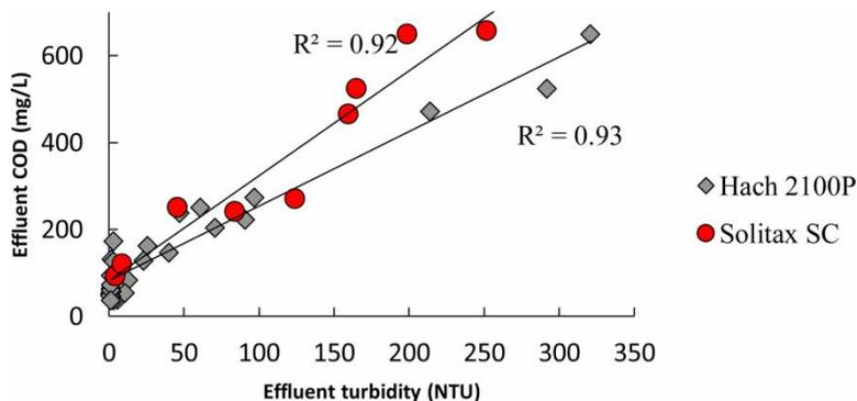
**Figure 4** | Correlations between effluent turbidity (NTU) and effluent COD (mg/L). Grab samples measured either online by the Solitax SC or with Hach Lange 2100P portable turbidity meter.
