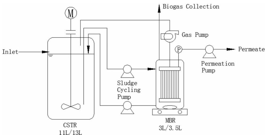
**Figure 1** | Flow diagram of the AnMBR system.
