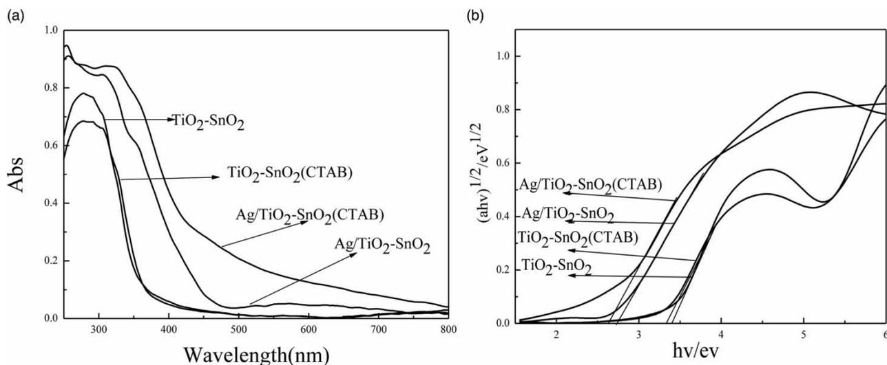
**Figure 2** | UV-vis-DRS of the as-synthesized samples (a) and the Kubelka-Munk energy curves of as-synthesized samples (b).
