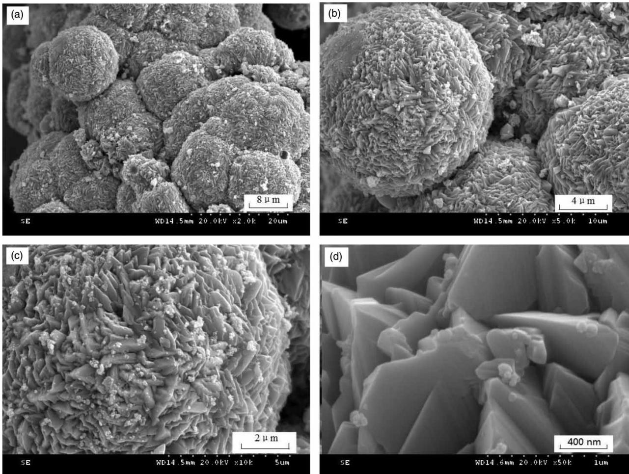
Figure 4 | SEM images of Ag/TiO<sub>2</sub>-SnO<sub>2</sub> (CTAB).
