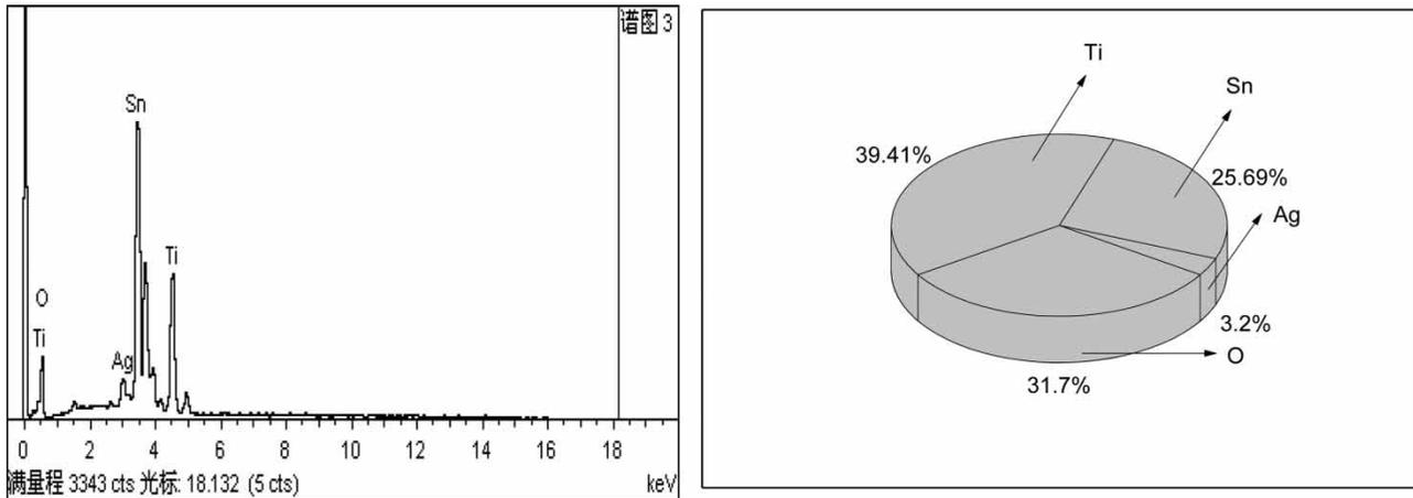
**Figure 6** | The EDS spectrum of as-synthesized Ag/TiO<sub>2</sub>-SnO<sub>2</sub> (CTAB) (left) and the actual element content in the as-synthesized Ag/TiO<sub>2</sub>-SnO<sub>2</sub> (CTAB) (right).
