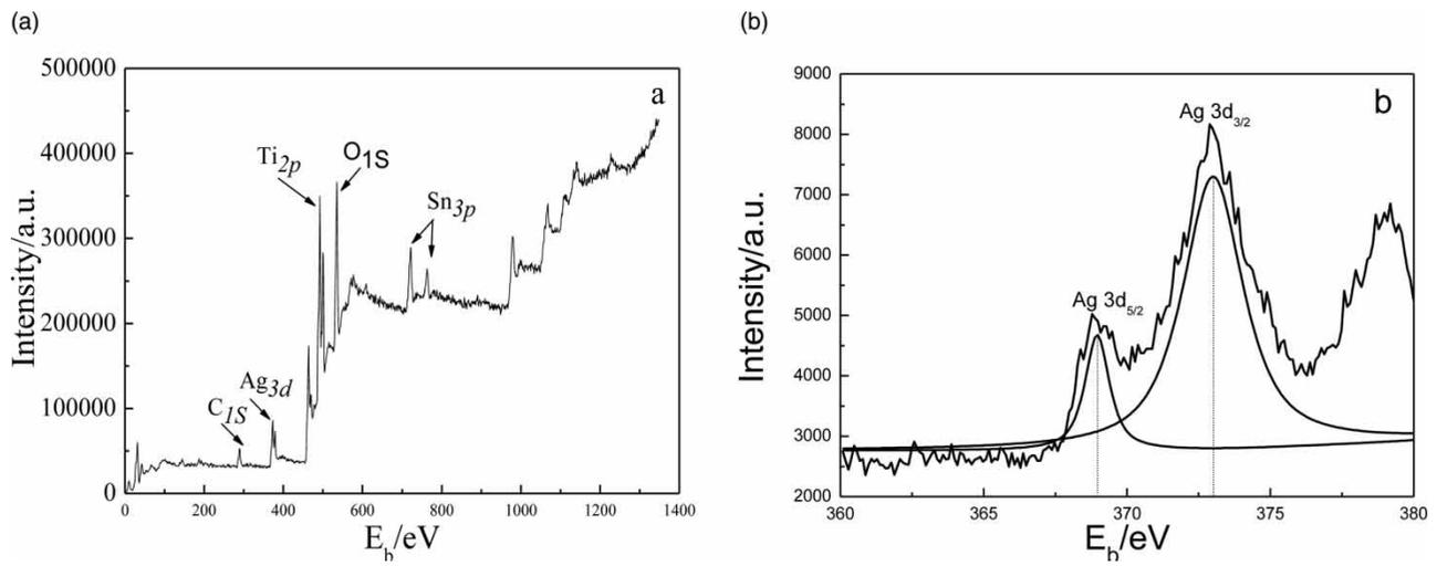
Figure 3 | The XPS spectrum of Ag/TiO<sub>2</sub>-SnO<sub>2</sub> (CTAB) (a) and the XPS spectra of Ag<sub>3d</sub> (b).
