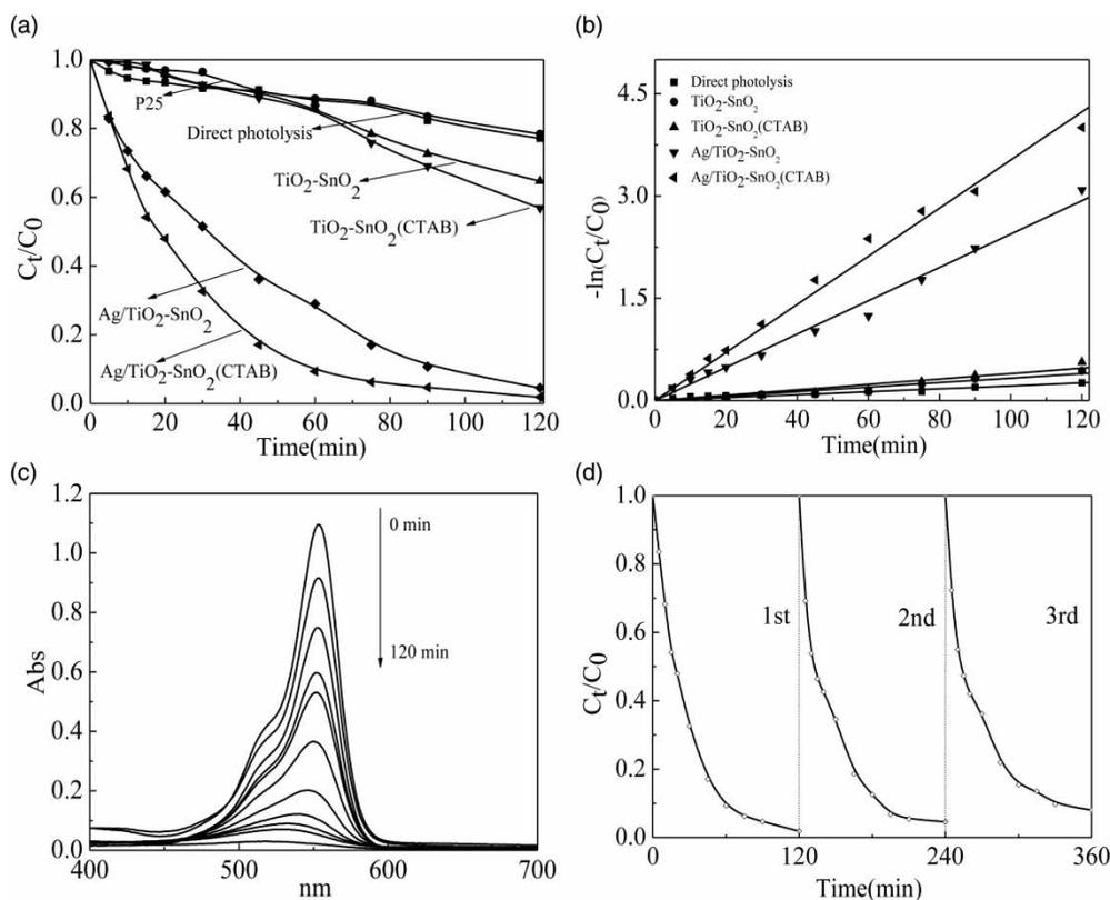
**Figure 8** | UV photocatalytic degradation of RhB using different photocatalysts (a), kinetics of UV photocatalytic degradation of RhB using different photocatalysts (b), UV photocatalytic degradation of RhB using Ag/TiO<sub>2</sub>-SnO<sub>2</sub> (CTAB) (c), and photocatalytic activities of Ag/TiO<sub>2</sub>-SnO<sub>2</sub> (CTAB) under UV irradiation for degradation of RhB after three cycles (d).
