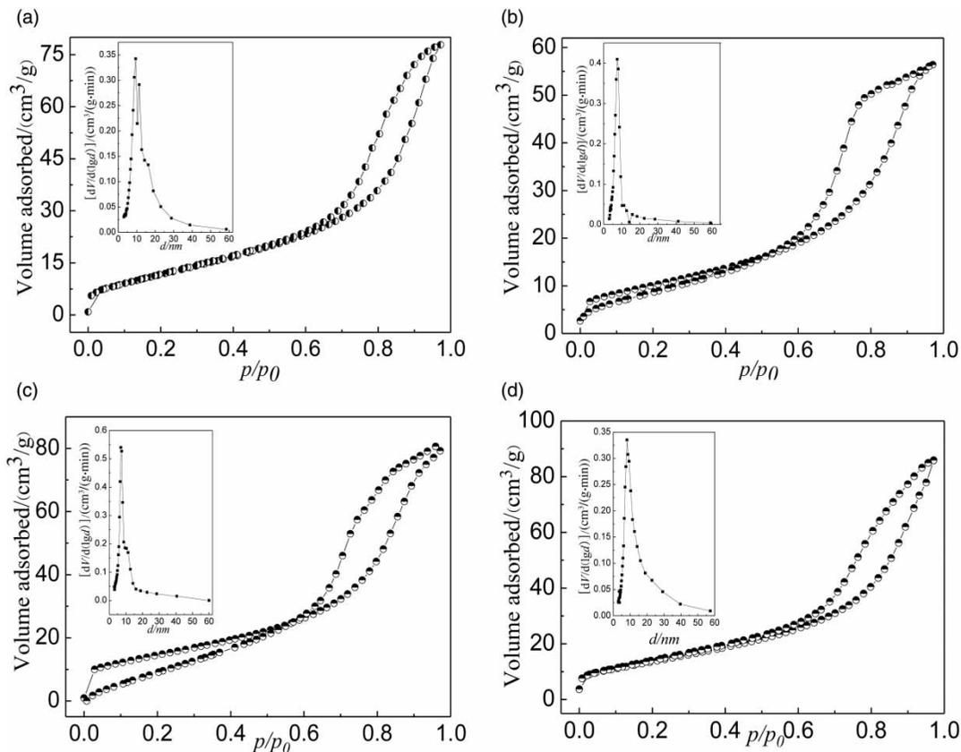
**Figure 7** | N<sub>2</sub> adsorption-desorption isotherms and pore size distribution curves of Ag/TiO<sub>2</sub>-SnO<sub>2</sub> (CTAB) (a), Ag/TiO<sub>2</sub>-SnO<sub>2</sub> (b), TiO<sub>2</sub>-SnO<sub>2</sub> (CTAB) (c), and TiO<sub>2</sub>-SnO<sub>2</sub> (d).
