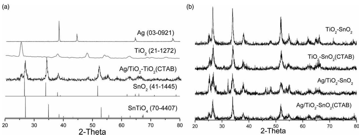
**Figure 1** | XRD patterns of Ag, TiO<sub>2</sub>, SnO<sub>2</sub>, SnTiO<sub>4</sub>, and as-synthesized Ag/TiO<sub>2</sub>-SnO<sub>2</sub> (CTAB) (a); XRD patterns of as-synthesized Ag/TiO<sub>2</sub>-SnO<sub>2</sub> (CTAB), Ag/TiO<sub>2</sub>-SnO<sub>2</sub>, TiO<sub>2</sub>-SnO<sub>2</sub>, and TiO<sub>2</sub>-SnO<sub>2</sub> (CTAB) (b).
