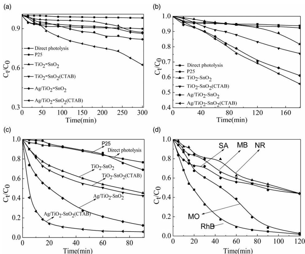
**Figure 9** | Photocatalytic degradation of RhB under simulated solar light (a), visible light (b), and microwave-assisted (c). Degradation of different organic pollutants by Ag/TiO<sub>2</sub>-SnO<sub>2</sub> (CTAB) under UV light (d).
