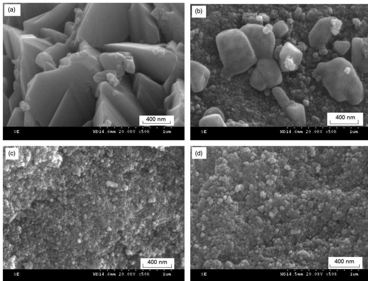
Figure 5 | SEM images of different products of Ag/TiO<sub>2</sub>-SnO<sub>2</sub> (CTAB) (a), Ag/TiO<sub>2</sub>-SnO<sub>2</sub> (b), TiO<sub>2</sub>-SnO<sub>2</sub> (CTAB) (c), and TiO<sub>2</sub>-SnO<sub>2</sub> (d).
