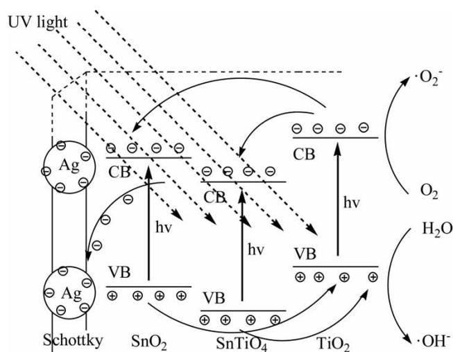
Figure 11 | Possible photocatalytic reaction mechanism of Ag/TiO<sub>2</sub>-SnO<sub>2</sub> (CTAB) composite.
