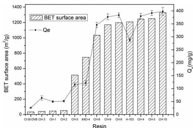
**Figure 2** | The curve of capacity vs BET surface area.
