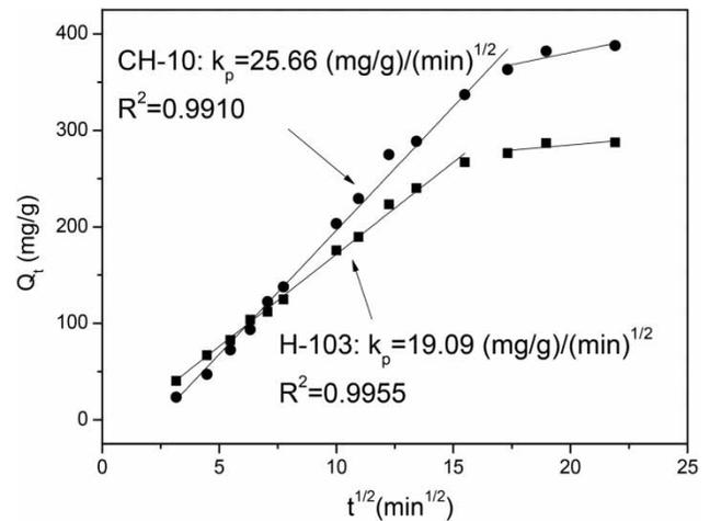
**Figure 6** | The relationship of  $Q_t$  vs  $t^{1/2}$  for the adsorption of nitrobenzene onto H-103 and CH-10 in aqueous solution at 303 K.
