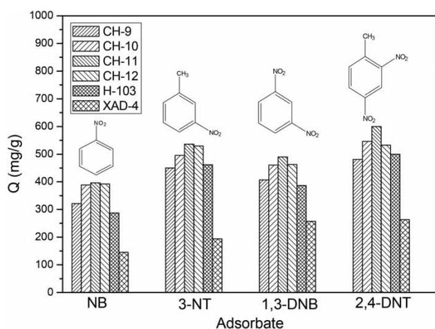
**Figure 8** | Adsorption capacity for nitroaromatics. Condition:  $C_0 = 100 \text{ mg/L}$ ;  $V = 0.2 \text{ L}$ ;  $m_{\text{(resin)}} = 20 \text{ mg}$ ;  $T = 303 \text{ K}$ ;  $t = 24 \text{ h}$ .
