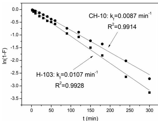
**Figure 5** | The straight lines of  $\ln(1-F)$  vs  $t$  for the adsorption of nitrobenzene onto H-103 and CH-10 in aqueous at 303 K.
