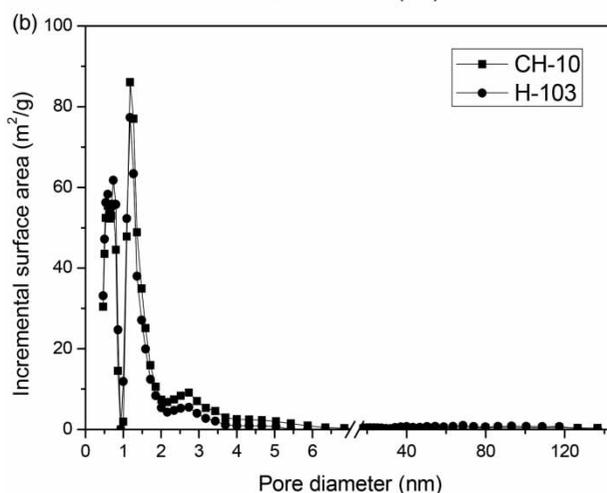
**Figure 3** | Pore size distribution vs incremental volume (a) and BET surface area (b) of H-103 and CH-10.
