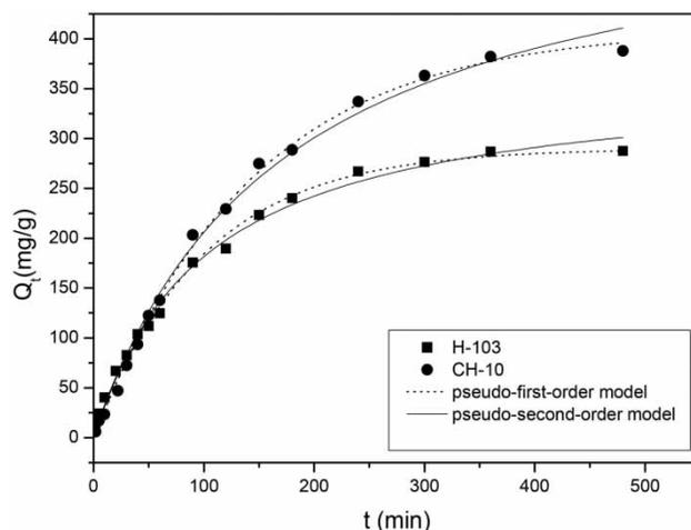
**Figure 4** | Adsorption kinetic curves of nitrobenzene onto CH-10 and H-103.
