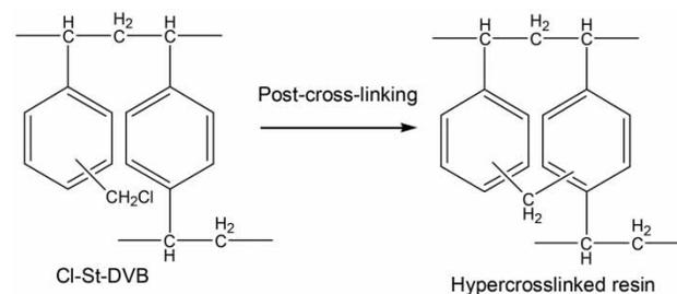
Figure 1 | Conceptual illustration of the synthetic procedure of hypercrosslinked resin (Pan *et al.* 2007).
