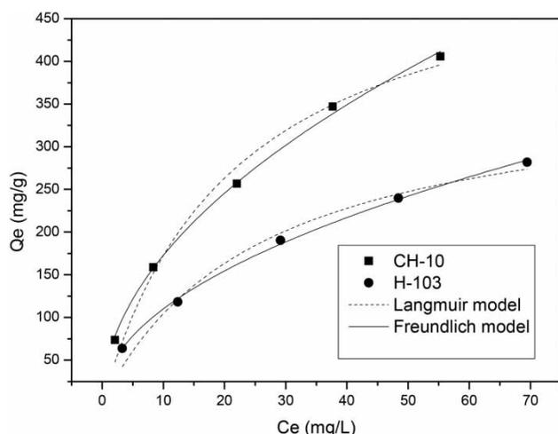
**Figure 7** | Adsorption isotherms of nitrobenzene adsorbed onto CH-10 and H-103 in aqueous solution at 303 K.
