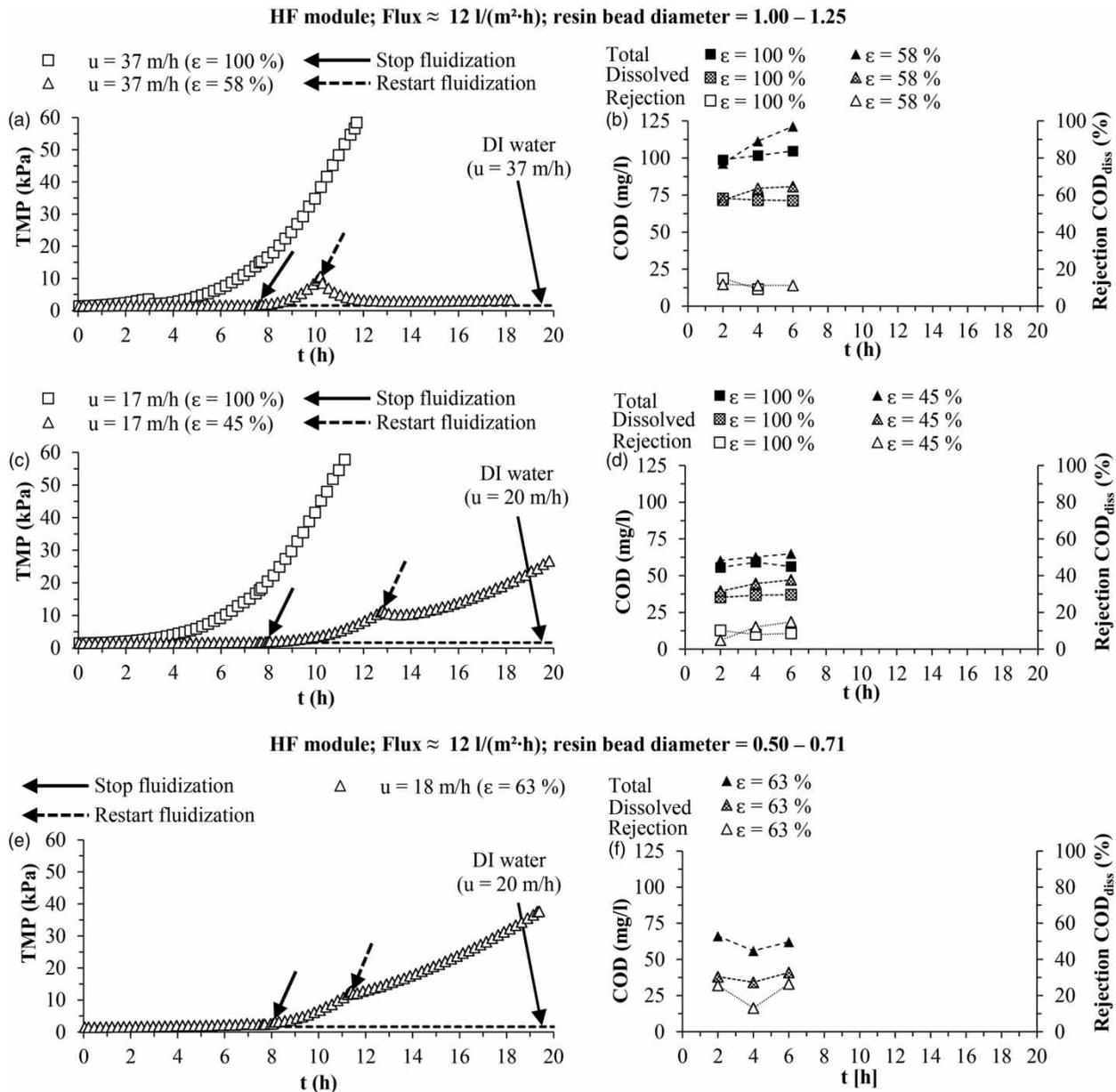
**Figure 3** | TMP during filtration of bioreactor effluent with HF module in the presence and absence ( $\epsilon = 100\%$ ) of fluidized resin beads (a), (c), (e).  $U$  is the crossflow velocity in the membrane module.  $\text{COD}_{\text{tot}}$  and  $\text{COD}_{\text{diss}}$  concentrations of the feed (inlet membrane module) and  $\text{COD}_{\text{diss}}$  rejection (b), (d), (f).
