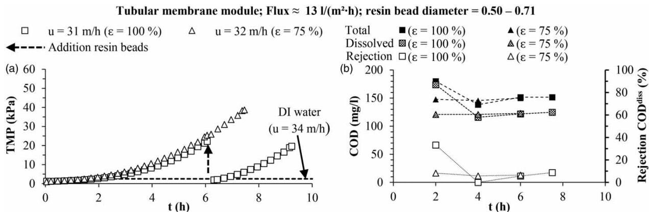
**Figure 2** | TMP during filtration of bioreactor effluent with tubular membrane in the presence and absence ( $\epsilon = 100\%$ ) of fluidized resin beads (a). After 6 hours, the empty-tube filtration test was stopped and resin beads were added (marked with arrow); a bed voidage of  $\epsilon = 75\%$  was adjusted.  $U$  is the crossflow velocity in the membrane module.  $COD_{tot}$  and  $COD_{diss}$  concentrations of the feed (inlet membrane module) and  $COD_{diss}$  rejection (b).
