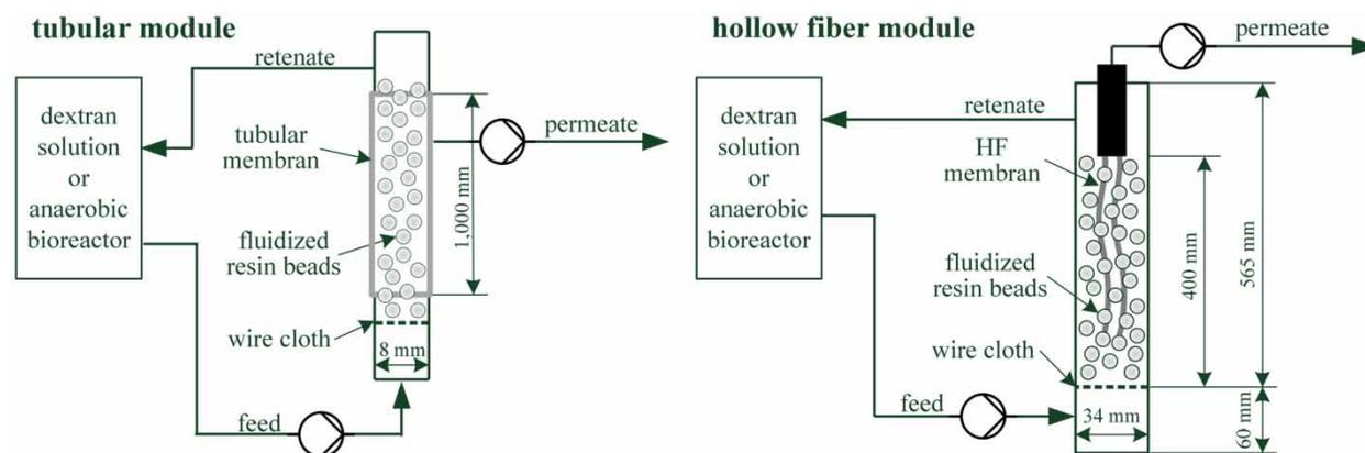
Figure 1 | Schematic diagram of the laboratory setups.
