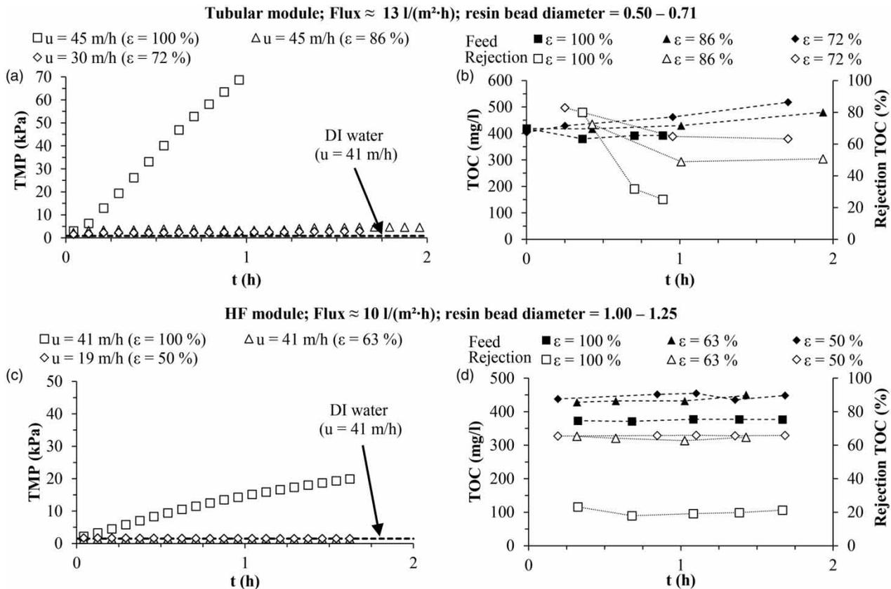
**Figure 4** | TMP increase during filtration ( $u$  = crossflow velocity) of dextran solution with tubular (a) and HF (c) membrane in the presence and absence ( $\epsilon = 100\%$ ) of fluidized resin beads. Total organic carbon (TOC) concentration of the feed (inlet membrane module) and TOC rejection (b) and (d).
