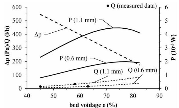
**Figure 5** | Predicted (theoretical) volume flow, pressure loss and required pumping power (HF membrane module) at filtration of bioreactor effluent. A mean particle diameter of 1.1 and 0.6 mm was assumed. Additionally, measured data for volume flow are shown (dots).
