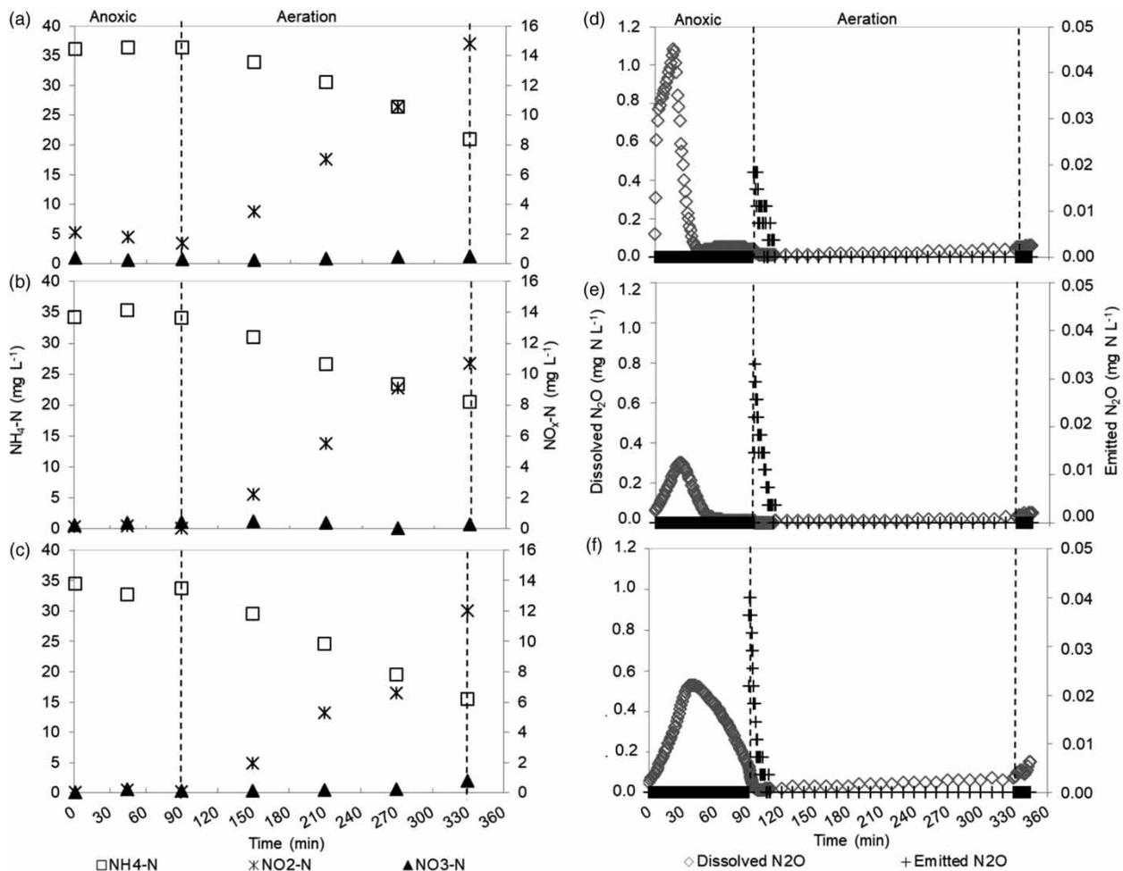
**Figure 3** | Bench-scale SBR operational cycle with AGS from the pilot system. During the 360 min cycle, the concentration profile of NH<sub>4</sub><sup>+</sup>-N, NO<sub>2</sub><sup>-</sup>-N and NO<sub>3</sub><sup>-</sup>-N and the effect of different COD/N ratios on N<sub>2</sub>O production/emission were monitored. (a) and (d) COD/N = 1.55; (b) and (e) COD/N = 1.17; (c) and (f) COD/N = 0.
