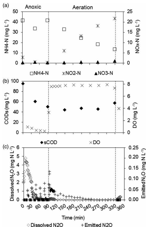
**Figure 2** | Pilot SBR operational cycle with AGS treating domestic wastewater. During the 360 min cycle, the concentration profile of NH<sub>4</sub><sup>+</sup>-N, NO<sub>2</sub><sup>-</sup>-N and NO<sub>3</sub><sup>-</sup>-N (a); COD and DO (b); and N<sub>2</sub>O production and emission (c) were measured over time.
