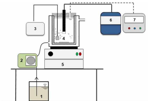
**Figure 1** | Bench experimental design. (1) Wastewater storage flask, (2) peristaltic pump, (3) compressed air, (4) bench reactor, (5) stirring table, (6) dissolved N<sub>2</sub>O sensor, (7) N<sub>2</sub>O gas sensor.
