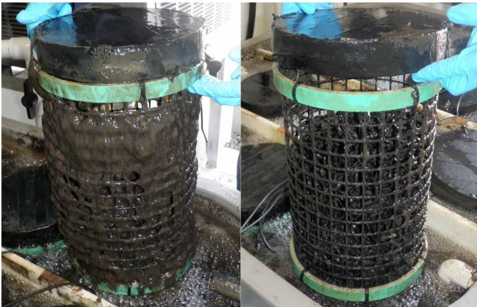
Figure 4 | Biofilm observed at 0.4 °C under a load of 6.6 g sCOD/m<sup>2</sup>.d (left) and 1.3 g sCOD/m<sup>2</sup>.d (right).
