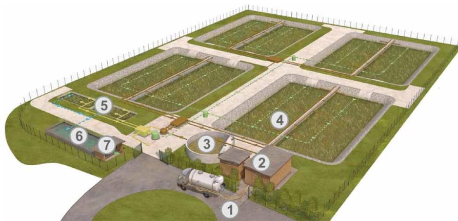
**Figure 1** | Schematic representation of the full scale STRB unit located in Nègrepelisse (Source: Epur Nature). (1) A septic tank emptying place, (2) a stone trap followed by automatic screening, (3) an aerated buffer tank, (4) eight STRB, (5) two VFCW, (6) a storage basin of treated leachate and (7) a filtration unit for irrigation.
