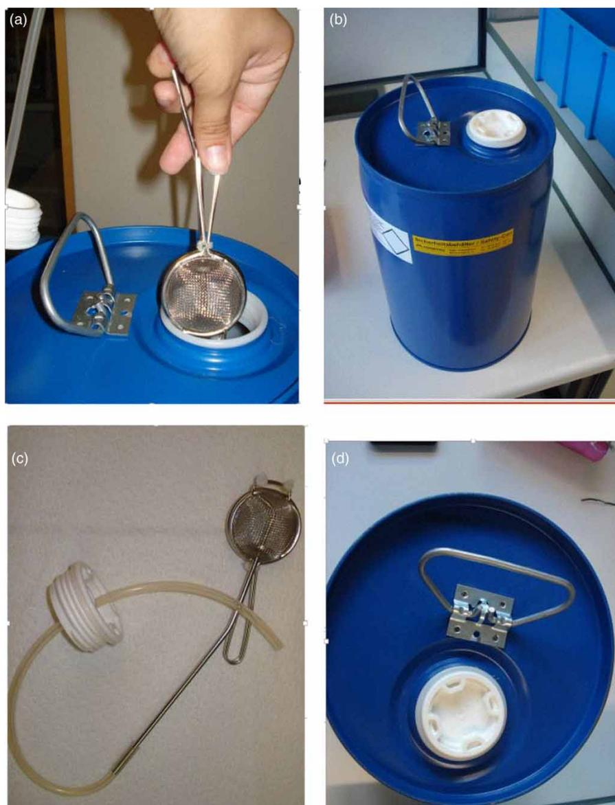
**Figure 1** | Set up of biodigester: (a) stainless steel container and PVC tube + metal sieve filtration unit + PVC lid, (b) stainless steel 15 L container, (c) full view of filtration unit, (d) biodigester top view.
