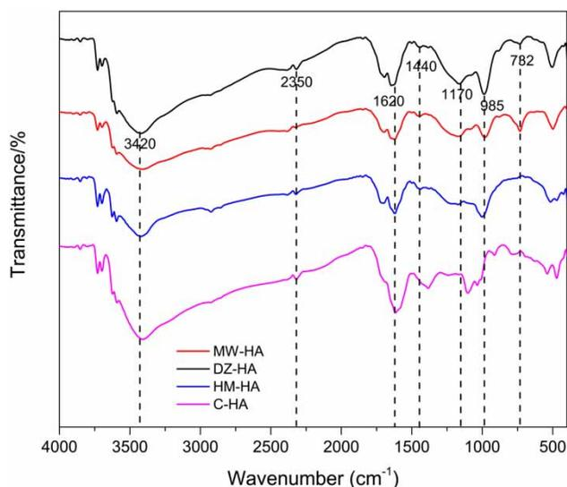
**Figure 1** | Comparison of FTIR spectra for HA samples.
