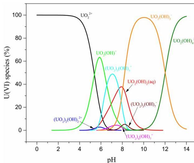
**Figure 3** | Effect of pH on speciation of U(VI) ( $T = 25\text{ }^{\circ}\text{C}$ ,  $C_{\text{U(initial)}} = 100\text{ }\mu\text{g L}^{-1}$ , ionic strength =  $0\text{ mol L}^{-1}$ ).
