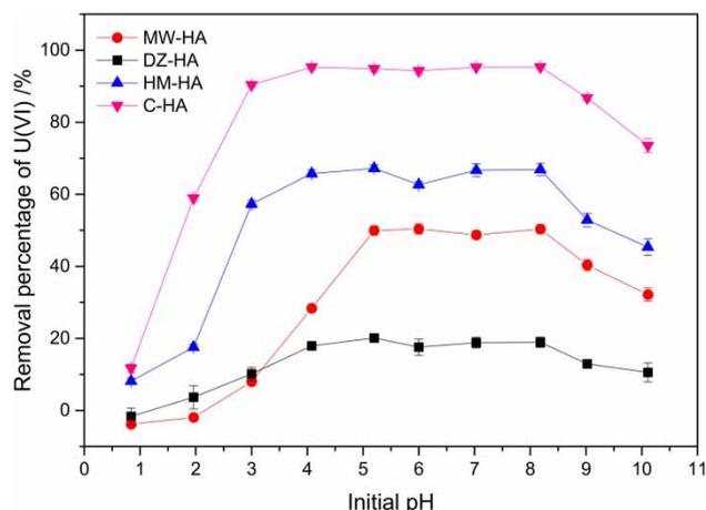
**Figure 2** | Effect of pH on U(VI) adsorption ( $T = 25\text{ }^{\circ}\text{C}$ ,  $C_{\text{U(initial)}} = 100\text{ }\mu\text{g L}^{-1}$ , ionic strength =  $0\text{ mol L}^{-1}$ ).
