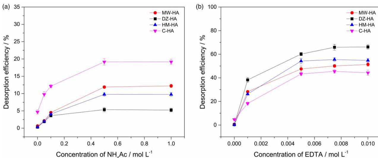
**Figure 7** | Desorption efficiency of uranium under the effect of  $\text{NH}_4\text{Ac}$  and EDTA.
