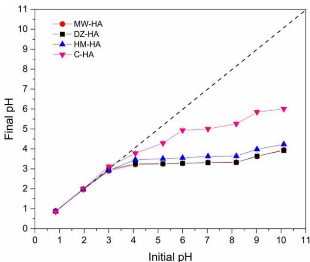
Figure 4 | The final pH of U(VI) solution.
