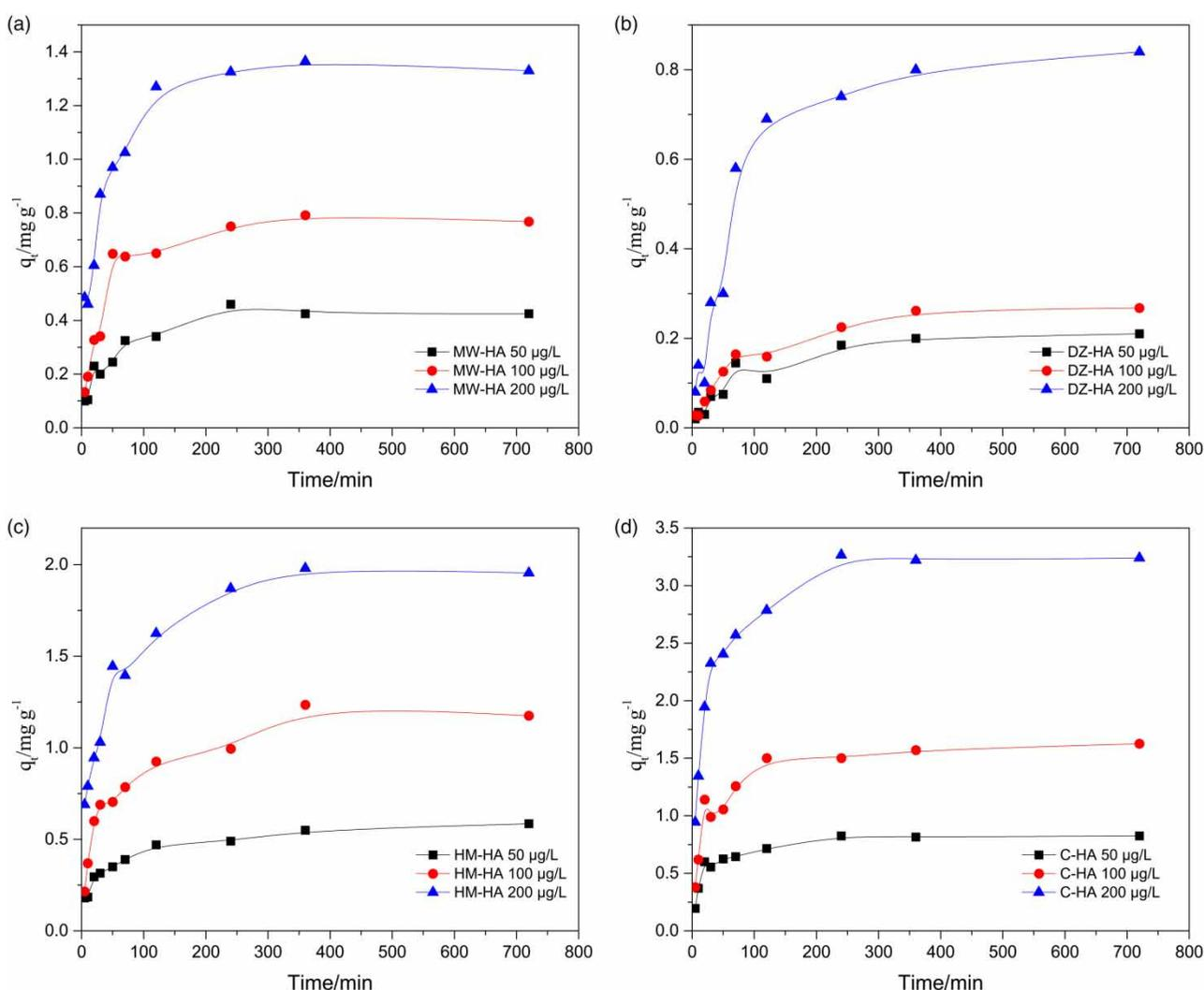
**Figure 6** | Effect of initial concentration on U(VI) adsorption: (a) MW-HA, (b) DZ-HA, (c) HM-HA, and (d) C-HA ( $T = 25\text{ }^{\circ}\text{C}$ ,  $\text{pH} = 5$ , ionic strength =  $0\text{ mol L}^{-1}$ ).
