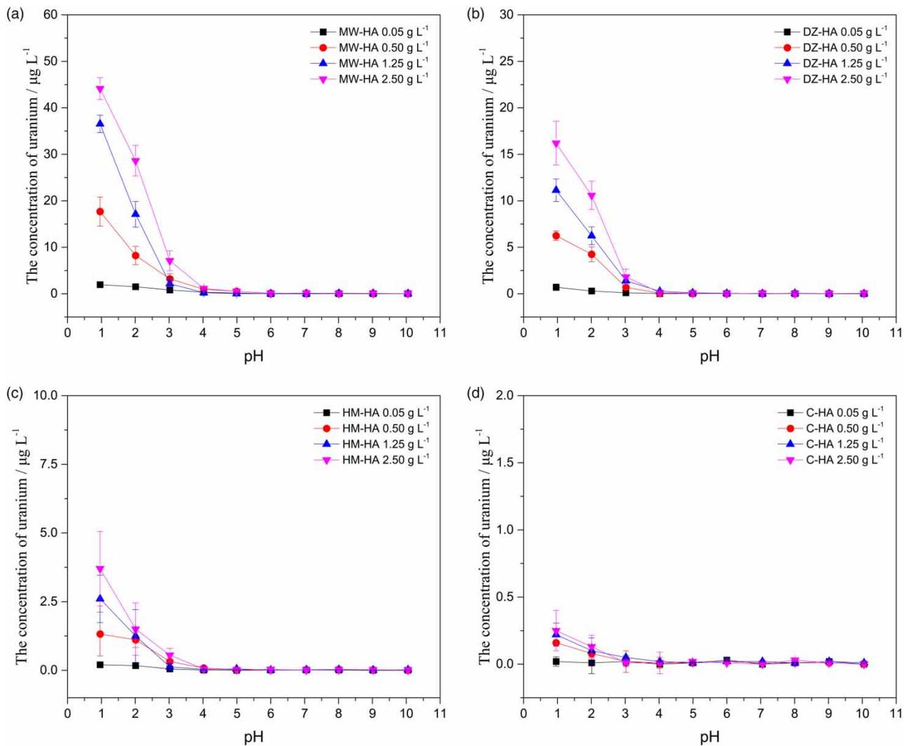
**Figure 5** | Effect of pH on uranium release from (a) MW-HA, (b) DZ-HA, (c) HM-HA and (d) C-HA ( $T = 25\text{ }^{\circ}\text{C}$ ,  $\text{pH} = 1\text{--}10$ , ionic strength =  $0\text{ mol L}^{-1}$ ).
