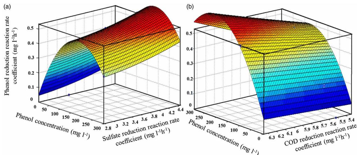
Figure 5 | Surface plots for (a) phenol and sulfate reduction reaction rate coefficients, and (b) phenol and COD reduction reaction rate coefficients with varied concentrations of phenol.
