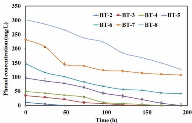
**Figure 2** | Time series plot of phenol reduction at different initial phenol concentrations.
