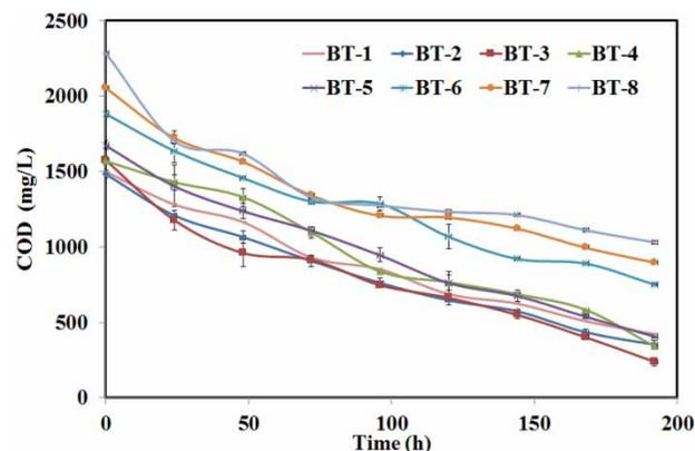
**Figure 3** | Time series plot of COD reduction at different initial phenol concentrations.
