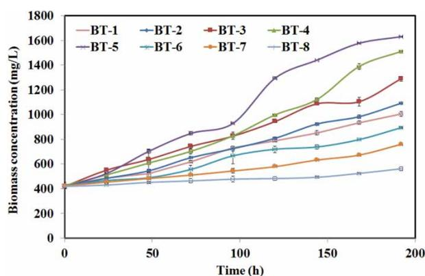
Figure 4 | Time series plot of biomass growth at different initial phenol concentrations.
