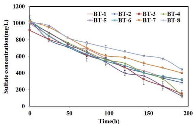
**Figure 1** | Time series plot of sulfate reduction at different initial phenol concentrations.
