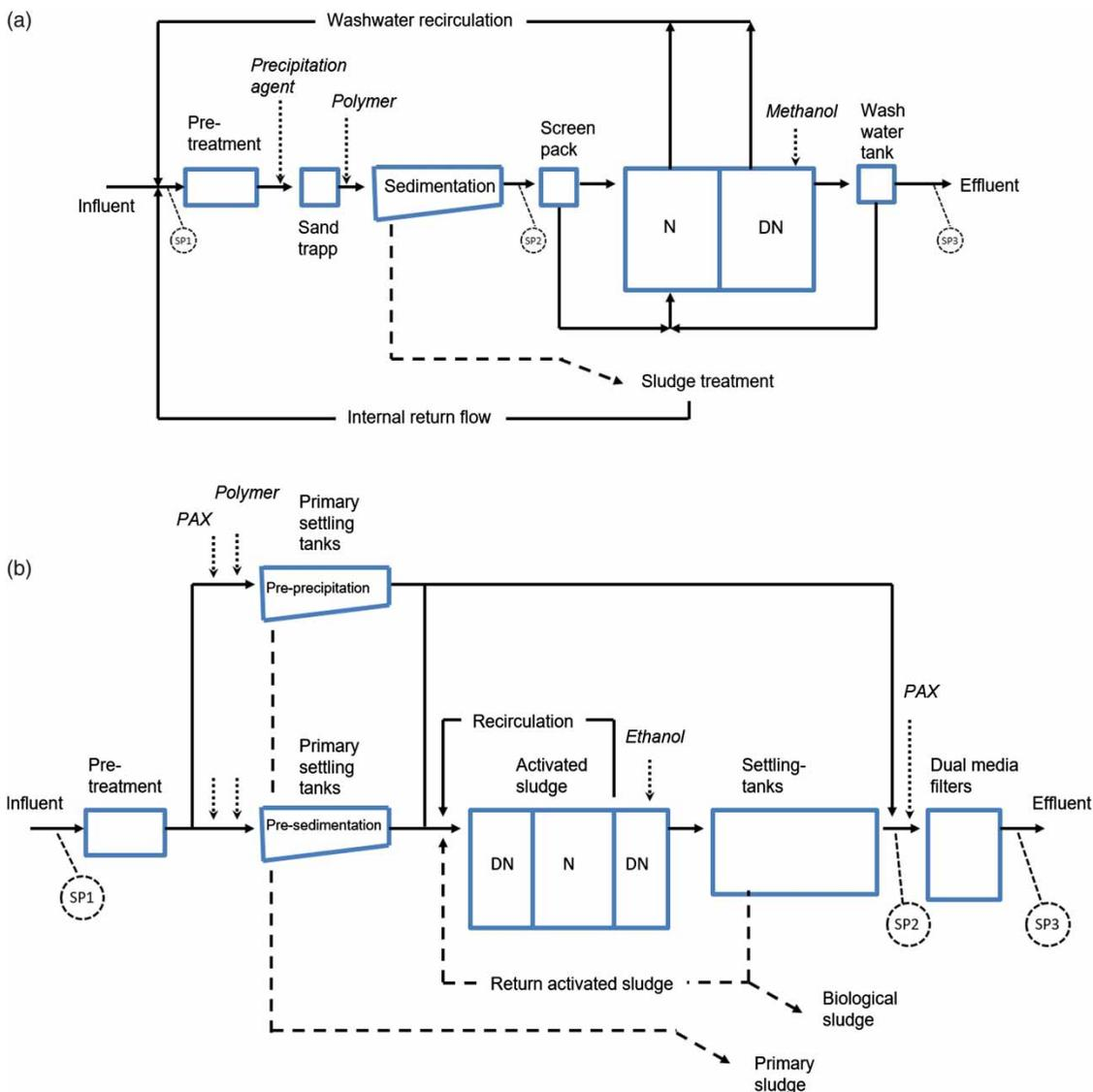
**Figure 1** | Simplified flow sheet of (a) VEAS and (b) BEVAS WWTPs. SP = Sampling point; N = Nitrification; DN = Denitrification (Figure b was adapted and modified from Storhaug 2014).
