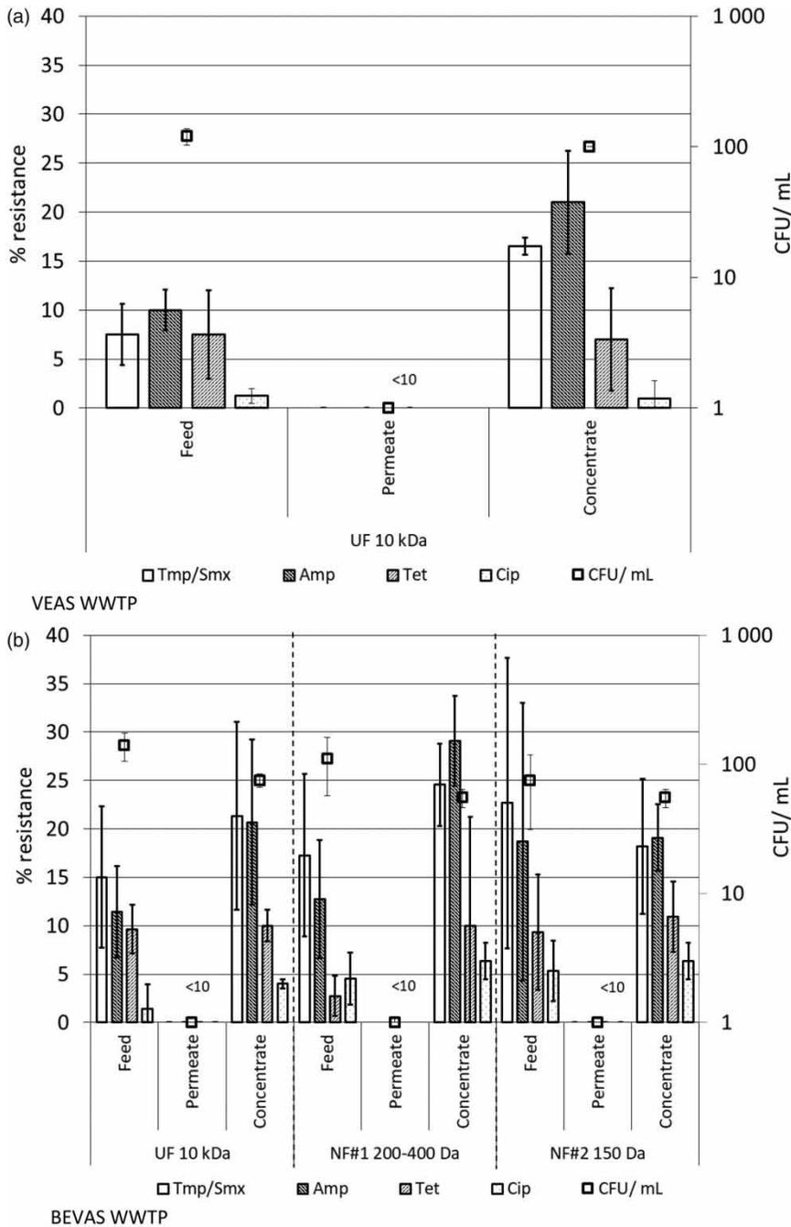
**Figure 5** | Concentrations of total viable *E. coli* (CFU/mL; boxes) and percentage (columns) of antibiotic resistant *E. coli* in the feed (i.e. WWTP effluent), permeate, and concentrate post-treatment with different membranes (UF = ultrafiltration; NF = nanofiltration). Feed samples were collected from (a) VEAS and (b) BEVAS WWTPs at different dates. Error bars represent 33% confidence interval (n = 2).
