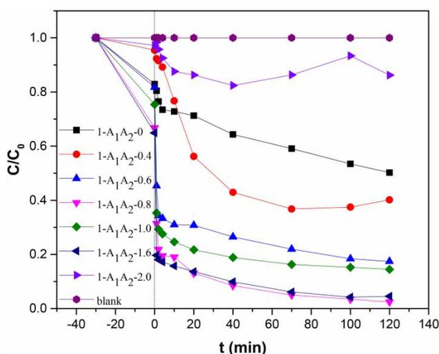
**Figure 4** | Photocatalytic activities of composites prepared with different amounts of CTAB for degradation of ciprofloxacin solution under visible light irradiation ( $\lambda > 420$  nm) at room temperature.
