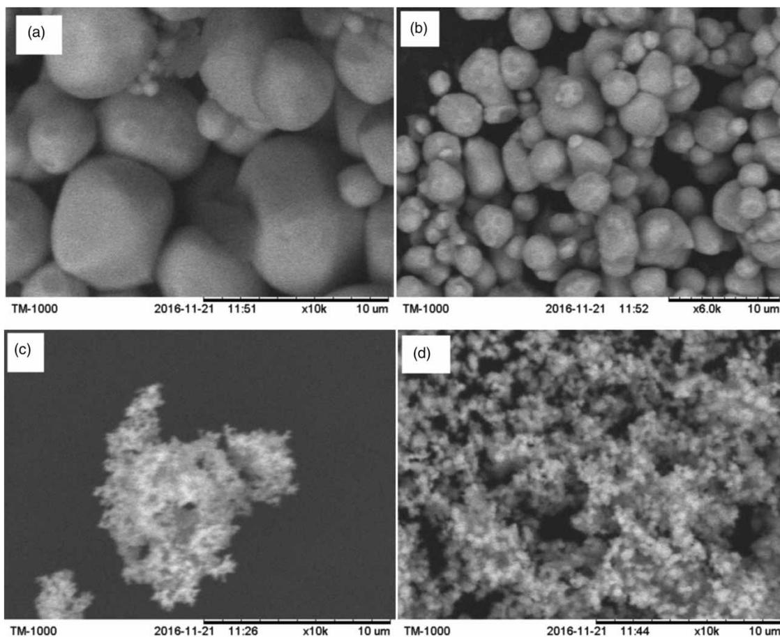
**Figure 1** | SEM images of  $\text{Ag}_3\text{PO}_4/\text{AgBr}$  products prepared with different amounts of CTAB: (a) 1- $\text{A}_1\text{A}_2$ -0.4, (b) 1- $\text{A}_1\text{A}_2$ -0.8, (c) 1- $\text{A}_1\text{A}_2$ -1.6, (d) 1- $\text{A}_1\text{A}_2$ -2.0.
