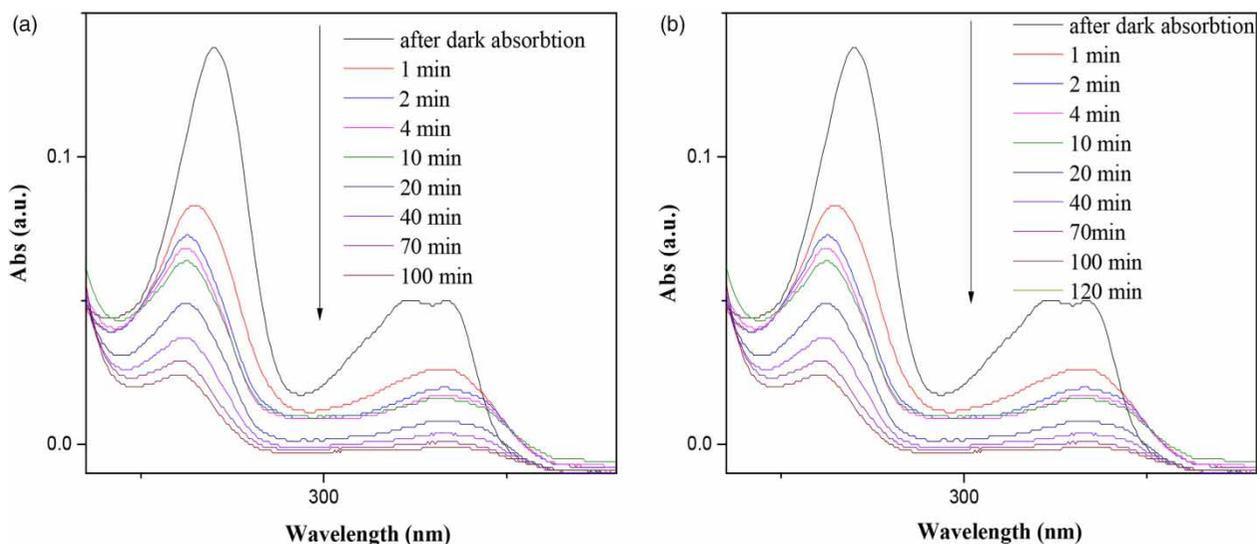
**Figure 5** | The absorption variation of ciprofloxacin solution over  $\text{Ag}_3\text{PO}_4/\text{AgBr}$  products at different irradiation time: (a) 1- $\text{A}_1\text{A}_2$ -1.0, (b) 1- $\text{A}_1\text{A}_2$ -0.6.
