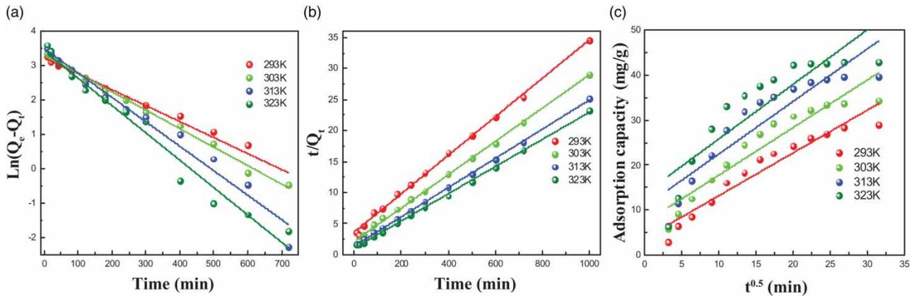
**Figure 6** | (a) Pseudo-first-order curves of Cd<sup>2+</sup> adsorption. (b) Pseudo-second-order curves of Cd<sup>2+</sup> adsorption. (c) Intra-particle diffusion model curves of Cd<sup>2+</sup> adsorption.
