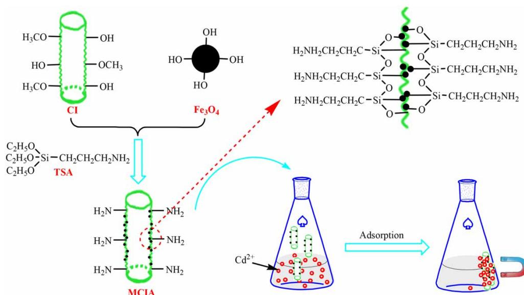
Figure 1 | The schematic preparation of bio-based magnetic adsorbent (MCIA) and application for Cd<sup>2+</sup> adsorption.
