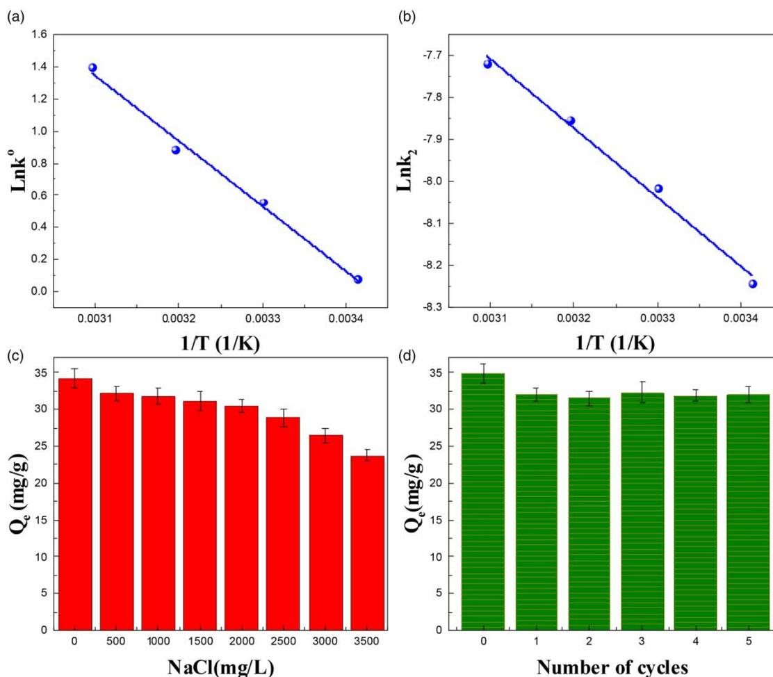
**Figure 8** | (a) The fitting of thermodynamic parameter for the uptake of cadmium ion. (b) The fitting of Arrhenius parameter at different temperature. (c) The effect of ionic strength for the adsorption capacities on the MCIA ( $T = 303$  K,  $\text{pH} = 6$ , initial concentration =  $40$  mg/L and contact time =  $12$  h). (d) Reusability of the MCIA for the  $\text{Cd}^{2+}$  uptake at  $303$  K and  $\text{pH} 6$ .
