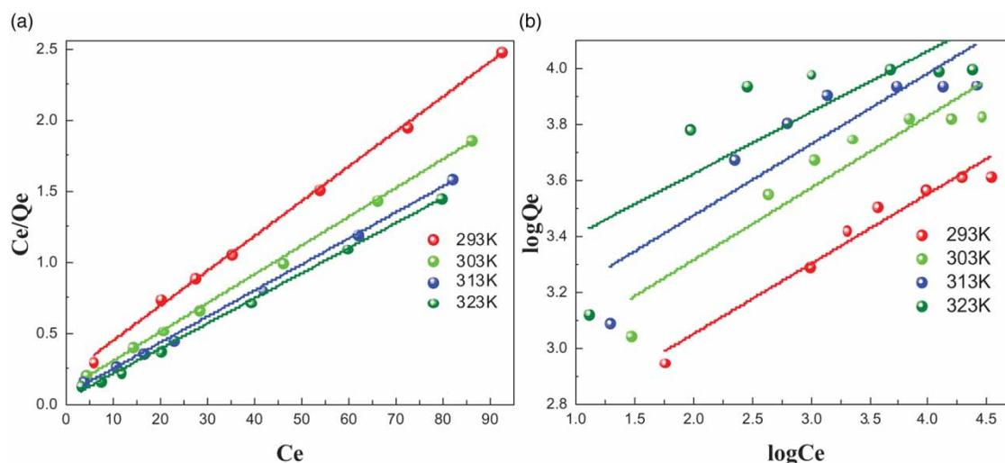
**Figure 7** | (a) The linear plots of Langmuir adsorption isotherm at different temperatures. (b) The linear plots of Freundlich adsorption isotherm at different temperatures.
