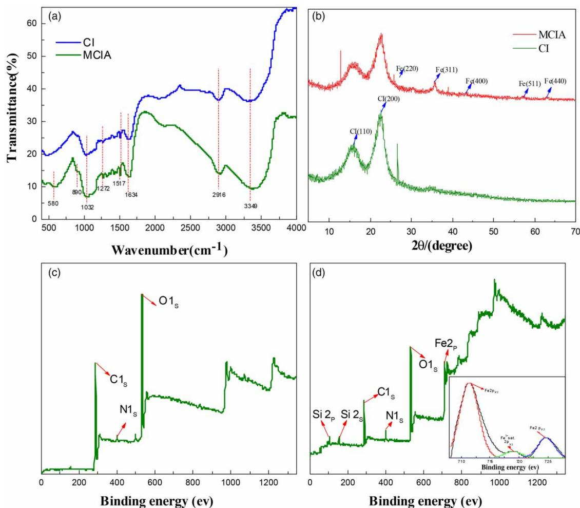
**Figure 2** | (a) The FTIR spectra of CI and MCIA. (b) The XRD spectra of CI and MCIA. The XPS spectra of CI (c) and MCIA (d).
