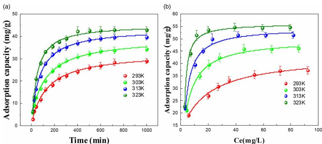
**Figure 5** | (a) The adsorption kinetics plot of MCIA for Cd<sup>2+</sup> at different temperature, pH = 6, concentration = 60 mg/L. (b) Effect of initial concentration on adsorption at different temperature, pH = 6.
