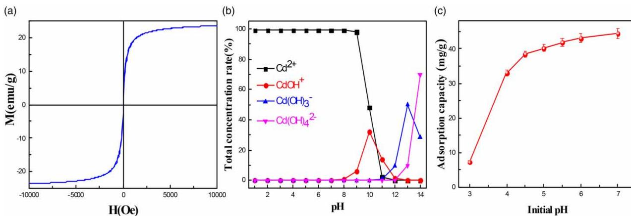
**Figure 4** | (a) The magnetization saturation curve for MCIA. (b) Species of cadmium ion at different pH (simulated by Visual MINTEQ 3.0). (c) Effect of pH on the adsorption of  $\text{Cd}^{2+}$  on MCIA at conditions of  $T = 303$  K, initial  $\text{Cd}^{2+}$  concentration = 60 mg/L, contact time = 12 h.
