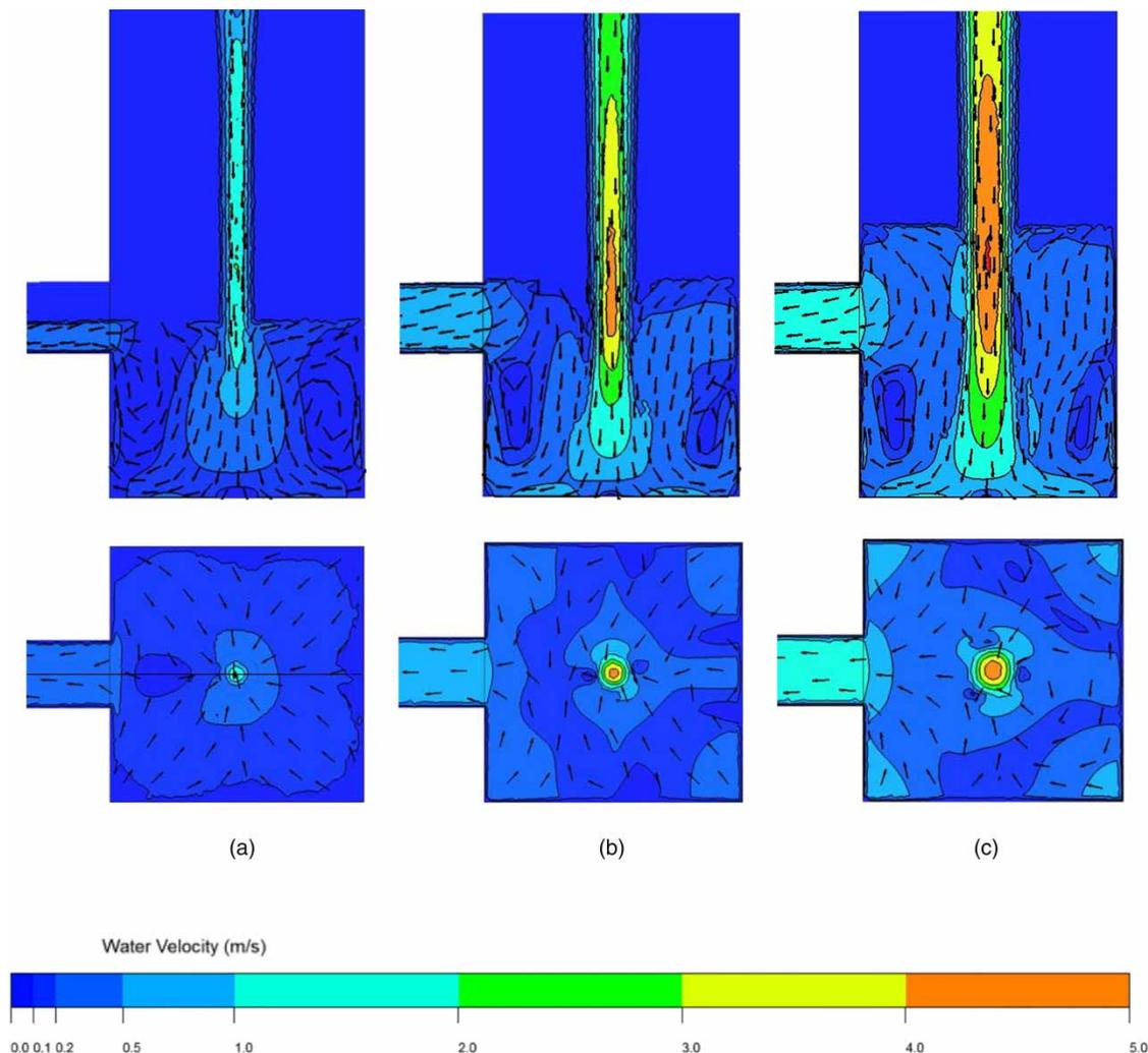
**Figure 4** | Water velocity vectors of the front view (center section) and top view at a level of 0.1 m above the outlet pipe invert for a flow rate of: (a) 7 L/s; (b) 28 L/s; (c) 56 L/s.
