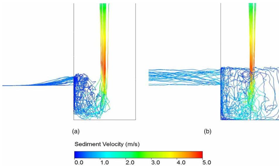
**Figure 5** | Trajectories of the escaped particles in the catch basin at a flow rate of 28 L/s (a) for particles of 1.8 mm, (b) 0.1 mm. Please refer to the online version of this paper to see this figure in color: <http://dx.doi.org/10.2166/wst.2018.009>.
