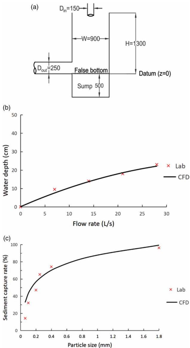
**Figure 1** | (a) Side view of the study catch basin of Tang *et al.* (2016); all dimensions are in mm). Comparisons of the simulations and the measurements of: (b) water depth and (c) sediment capture rates at a flow rate of 28 L/s.
