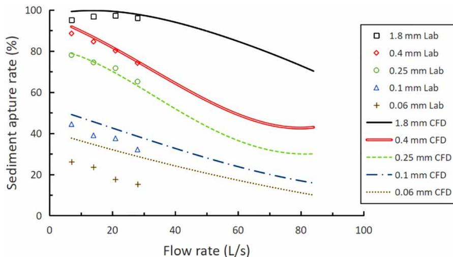
**Figure 3** | CFD predicted sediment capture rate compared with the measurements of Tang *et al.* (2016) for different particle sizes.
