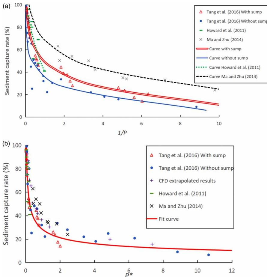
Figure 7 | Sediment capture rate (a) as a function of  $1/P$ , (b) as a function of  $P^*$ .
