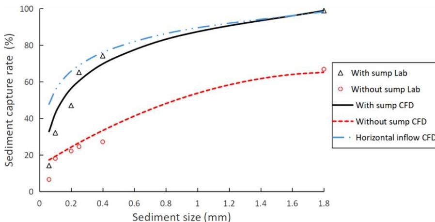
**Figure 6** | Sediment capture rates in different catch basin structures at a flow rate of 28 L/s.
