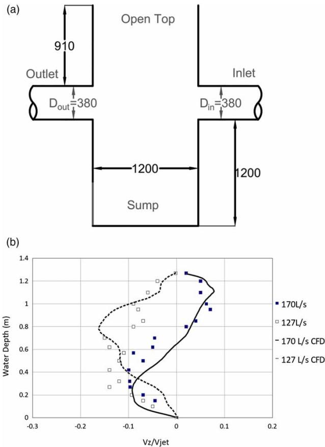
**Figure 2** | (a) Side view of the experimental setup of Howard *et al.* (2011); all dimensions are in mm. (b) Distribution of the normalized vertical velocity at two flow rates. Measurements were taken at 0.4 m upstream of the outlet in the center plane.
