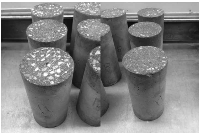
Figure 3 | Top and bottom of cylinders with w/c ratio 0.67.
