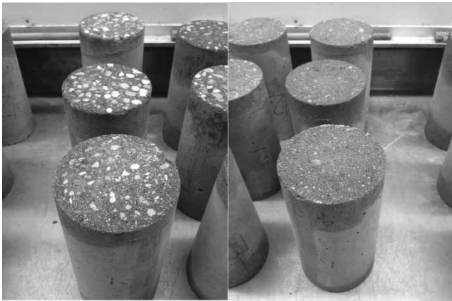
Figure 2 | Top and bottom of cylinders with w/c ratio 0.76.
