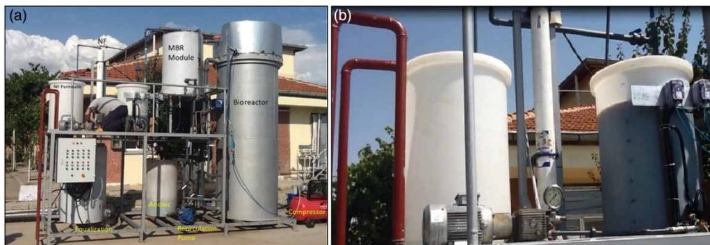
Figure 2 | Pictures of (a) pilot plant and (b) membrane units – MBR/NF.
