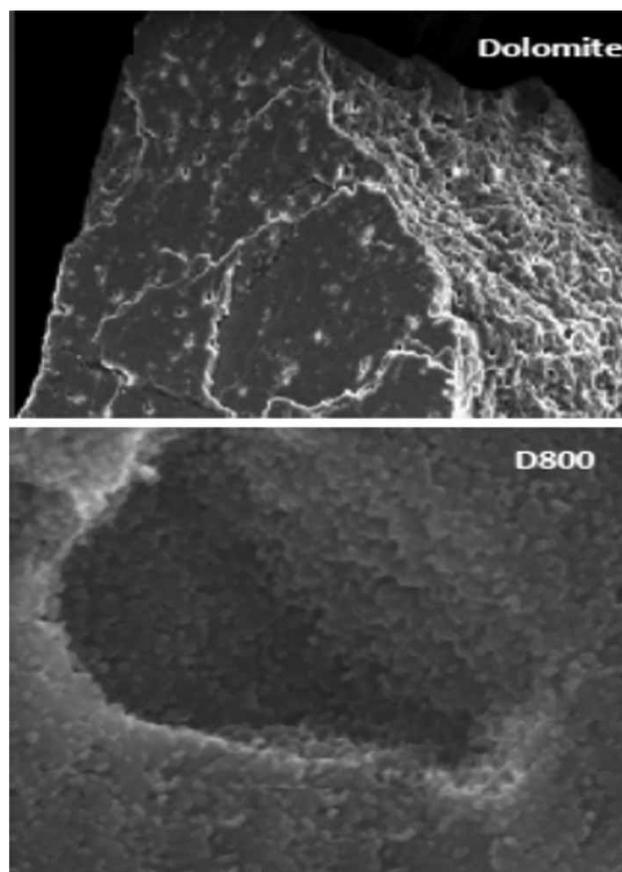
**Figure 2** | SEM images of dolomite and D800.
