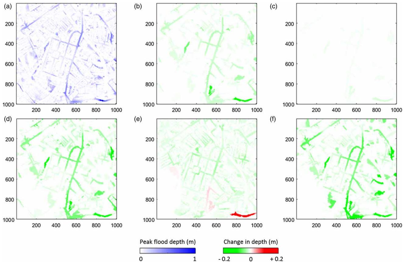
**Figure 5** | Peak flood depths during a one-hour 200-year return period rainfall event: (a) do nothing, (b) green roof, (c) water butt, (d) rainwater re-use, (e) permeable paving and (f) upgrade drainage. Please refer to the online version of this paper to see this figure in colour: <http://dx.doi.org/10.2166/wst.2018.122>.
