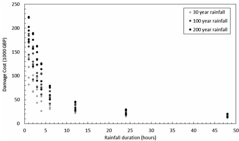
**Figure 4** | Catchment critical rainfall duration identified using a damage assessment for all interventions during 30-, 100- and 200-year rainfall events (144 simulations).
