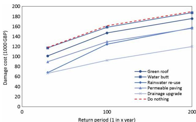
**Figure 7** | Damage cost versus increasing rainfall intensity during the two-hour rainfall event.
