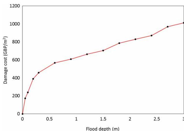
**Figure 3** | Flood depth damage curve for a typical three-bedroom semi-detached property (Penning-Orswell *et al.* 2010).
