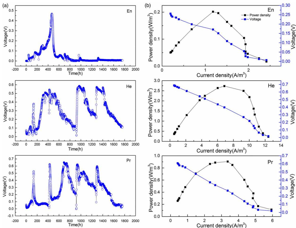
**Figure 1** | Voltage changes (a) and power density and polarization curves (b) in MFCs fed with the activated sludge pretreated by thermophile (En), 100 °C heating (He) and 121 °C heating (Pr).
