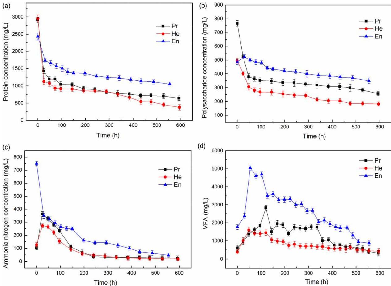
**Figure 3** | Changes of protein (a), polysaccharide (b), ammonia nitrogen (c) and volatile fatty acids (VFAs) (d) in the anode chambers of MFCs fed with the activated sludge pretreated by thermophile (En), 100 °C heating (He) and 121 °C heating (Pr).
