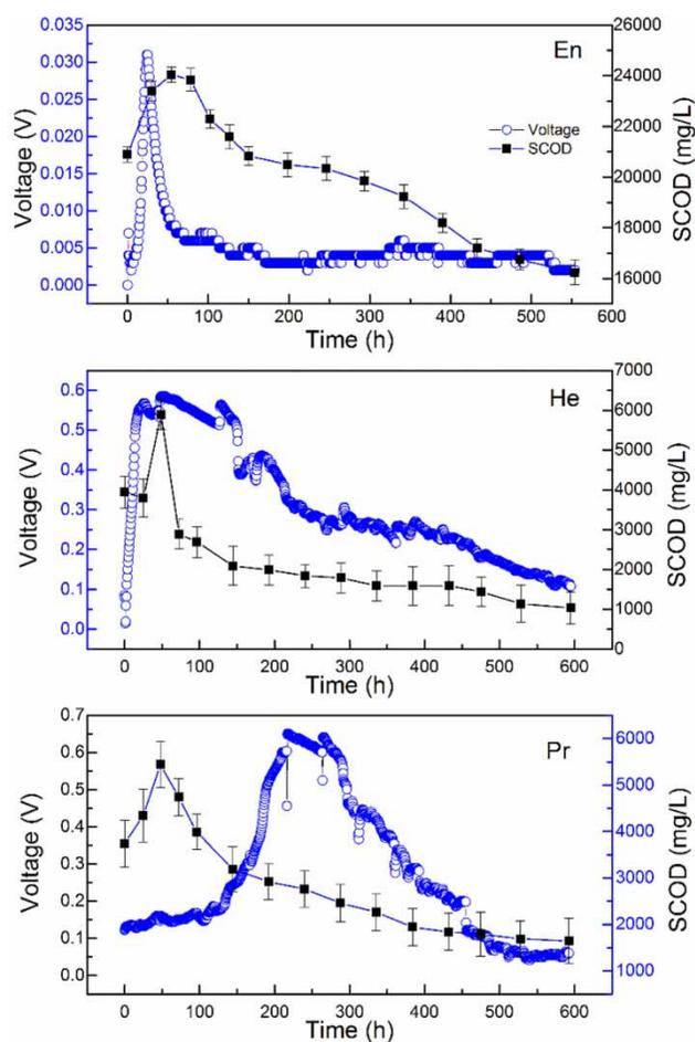
**Figure 2** | Voltage and SCOD changes in MFCs fed with the activated sludge pretreated by thermophile (En), 100 °C heating (He) and 121 °C heating (Pr) in one feeding cycle.
