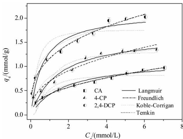
**Figure 5** | Adsorption isotherms for the adsorption of CA, 4-CP and 2,4-DCP on GPAC at 298 K.
