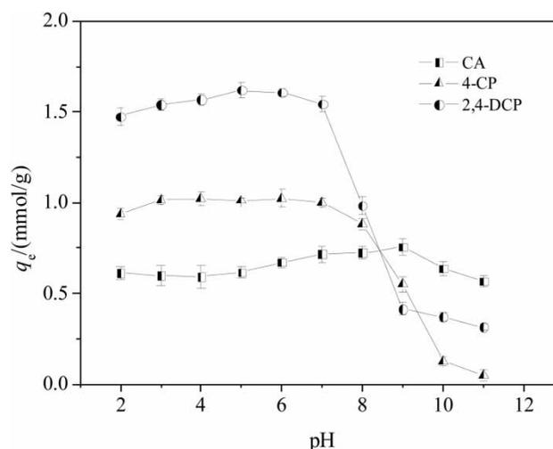
Figure 3 | Effect of initial pH on the removal of phenolic compounds by GPAC.
