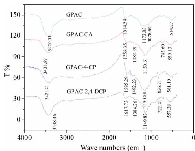
**Figure 1** | FTIR spectra of GPAC and GPAC-adsorbed CA, 4-CP and 2,4-DCP.
