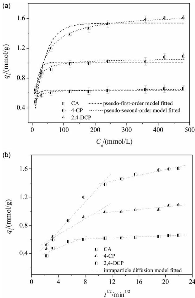
**Figure 4** | Pseudo-first-order and pseudo-second-order (a) and intraparticle diffusion (b) models for the adsorption of phenolic compounds on GPAC ( $C_0$  (CA, 4-CP, 2,4-DCP) = 4 mmol/L).
