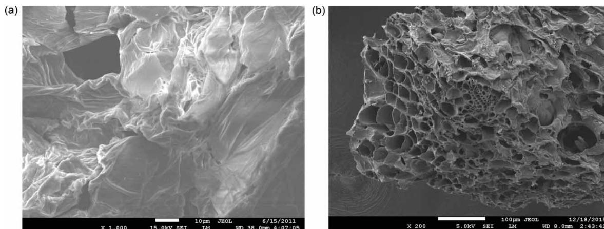
**Figure 2** | SEM image of (a) grapefruit peel and (b) GPAC.
