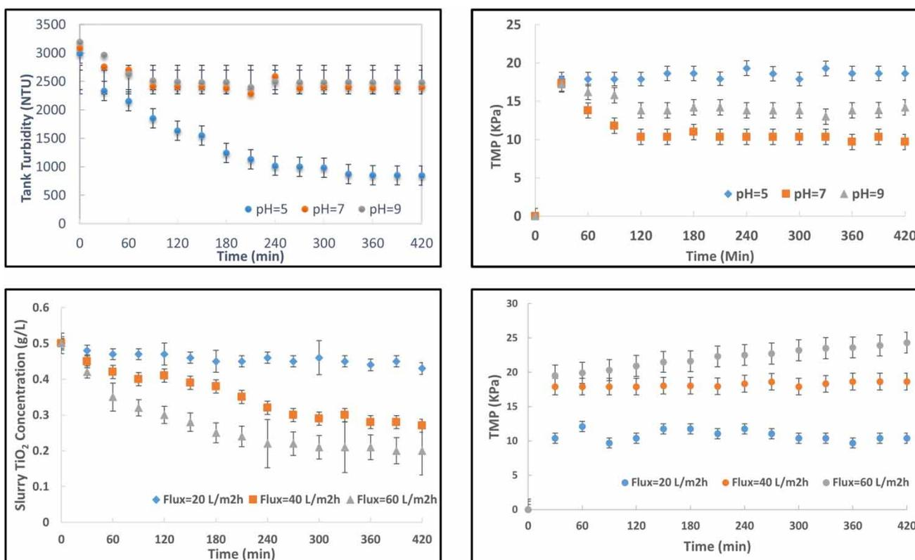
**Figure 7** | Effect of pH – measured in terms of (a) tank turbidity and (b) TMP and effect of permeate flux – measured in terms of (c) slurry  $\text{TiO}_2$  concentrations and (d) TMP on membrane fouling. The error bars denote standard deviation.
