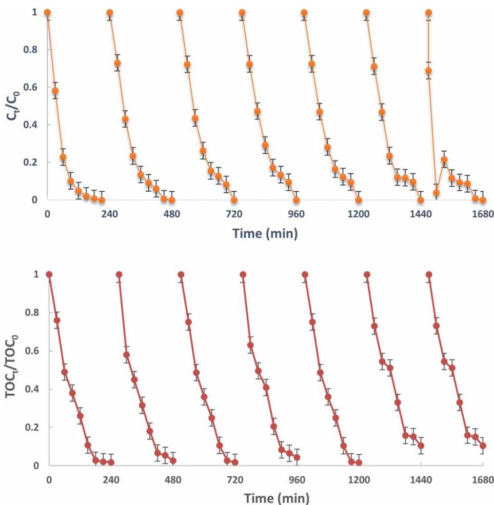
**Figure 2** | Performance of PMR on (a) PHE removal and (b) TOC removal during seven cycles of catalyst reuse ([PHE] = 1,000  $\mu\text{g/L}$ ,  $[\text{TiO}_2]$  = 0.5 g/L, pH = 7, n = number of cycles). The error bars denote standard deviation.
