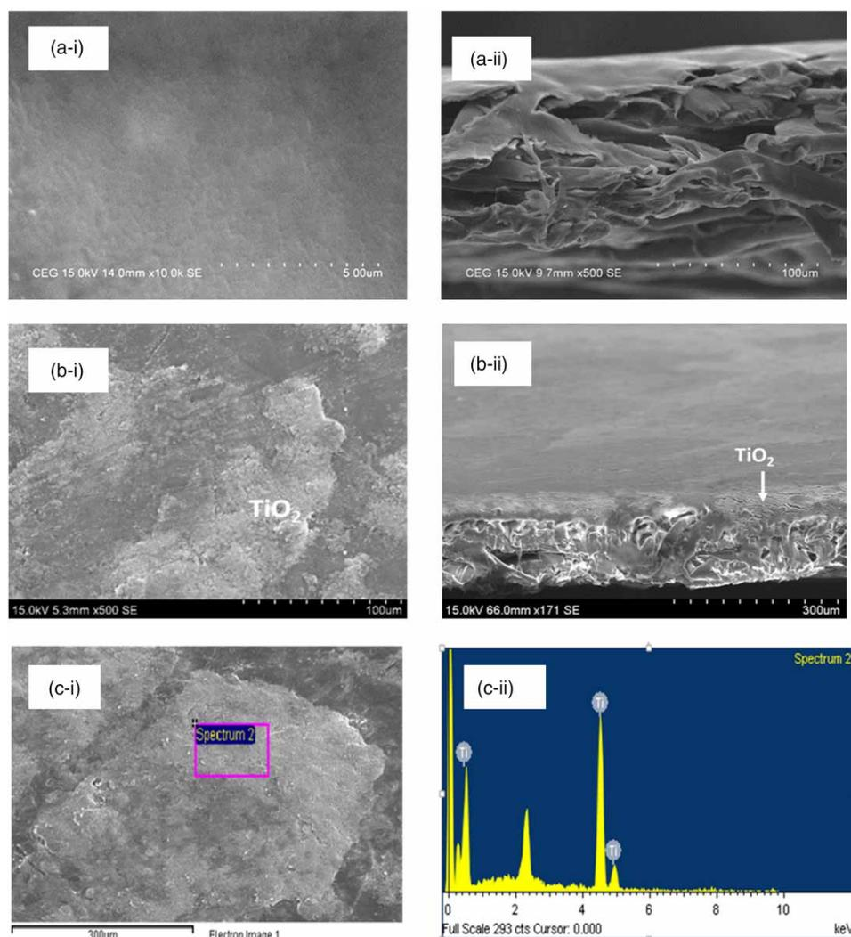
**Figure 6** | SEM images of the (a) clean (i) top view and (ii) cross sectional view, (b) used membrane (i) top view and (ii) cross sectional view and (c) (i) and (ii) SEM with EDS image.
