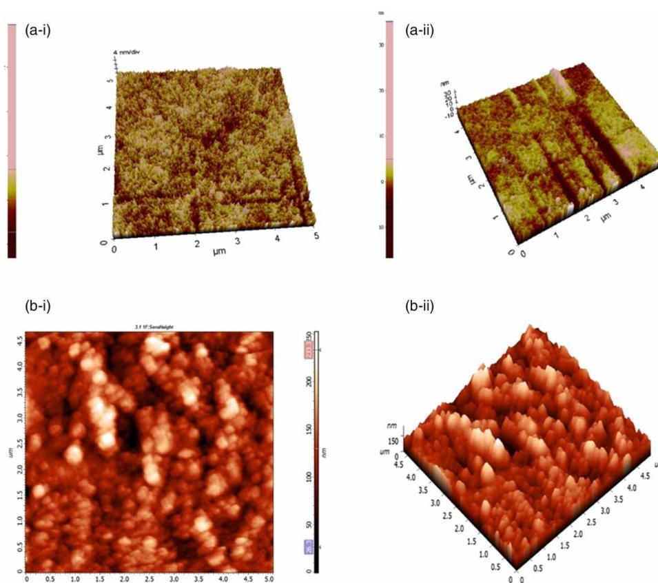
**Figure 5** | AFM images of (a) clean (i) two dimensional image, (ii) three dimensional image and (b) used membrane (i) two dimensional image, (ii) three dimensional image.
