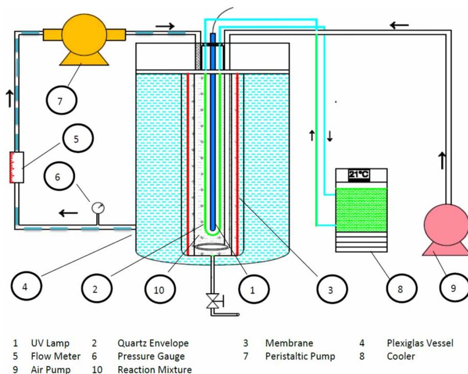
Figure 1 | Experimental setup of photocatalytic membrane reactor.
