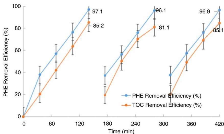
**Figure 3** | Performance of slurry PMR in continuous mode ([PHE] = 1,000 µg/L, TiO<sub>2</sub> = 0.5 g/L). The error bars denote standard deviation.
