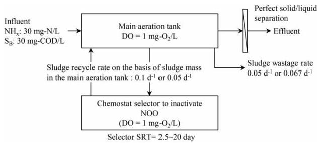
Figure 4 | Simulation boundary of NOO washout using selector.
