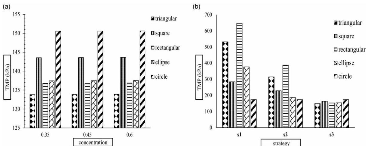
Figure 9 | TMP changes via concentration in S3 (a). Comparison of the TMP in all considered geometries and strategies by reducing the HF number (b).
