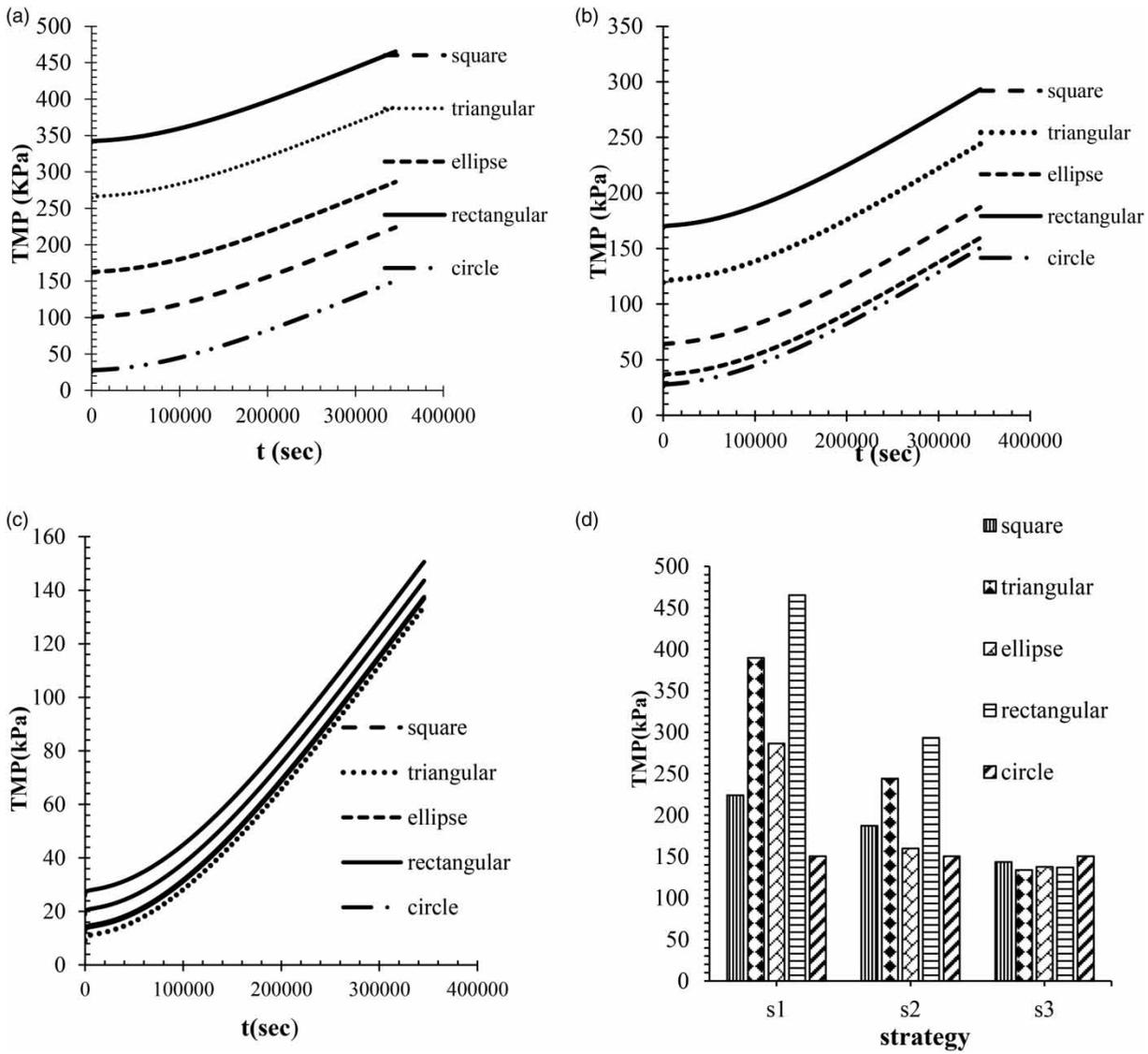
Figure 6 | Comparison of TMP changes in all geometries in S1 (a), S2 (b) and S3 (c), and maximum TMP for all geometries in all strategies (d).
