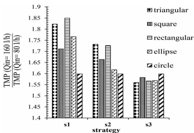
**Figure 10** | The TMP variations by 50% reduction of the feed flow rate.
