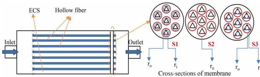
Figure 2 | Cross-section of triangle inner shape HF membrane in S1, S2, and S3.
