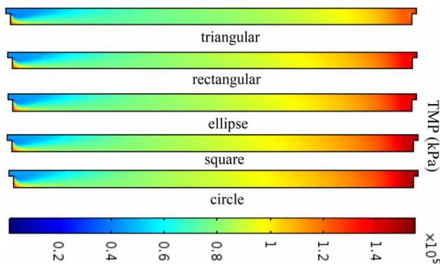
Figure 7 | Comparison of the pressure difference between ECS and lumen and TMP in the S3 for all considered geometries.
