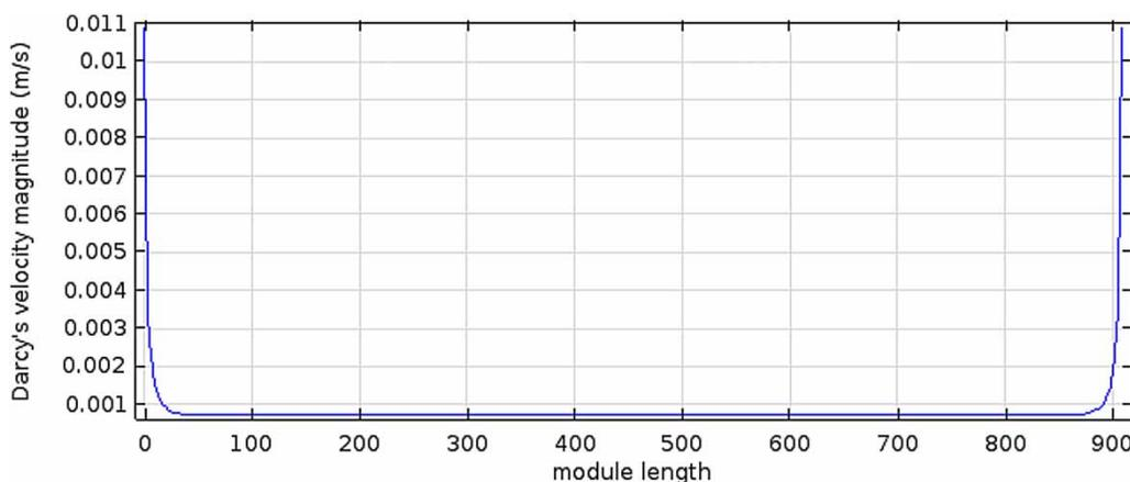
Figure 5 | The Darcy's velocity magnitude in the module.
