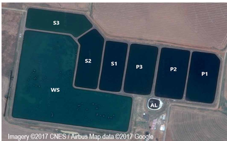
Figure 1 | Western Waters' Bacchus Marsh Recycled Water Plant. Aerobic lagoon (AL), primary lagoons (P1–P3), secondary lagoons (S1–3) and winter storage lagoon (WS) ( Google Maps 2017 ).
