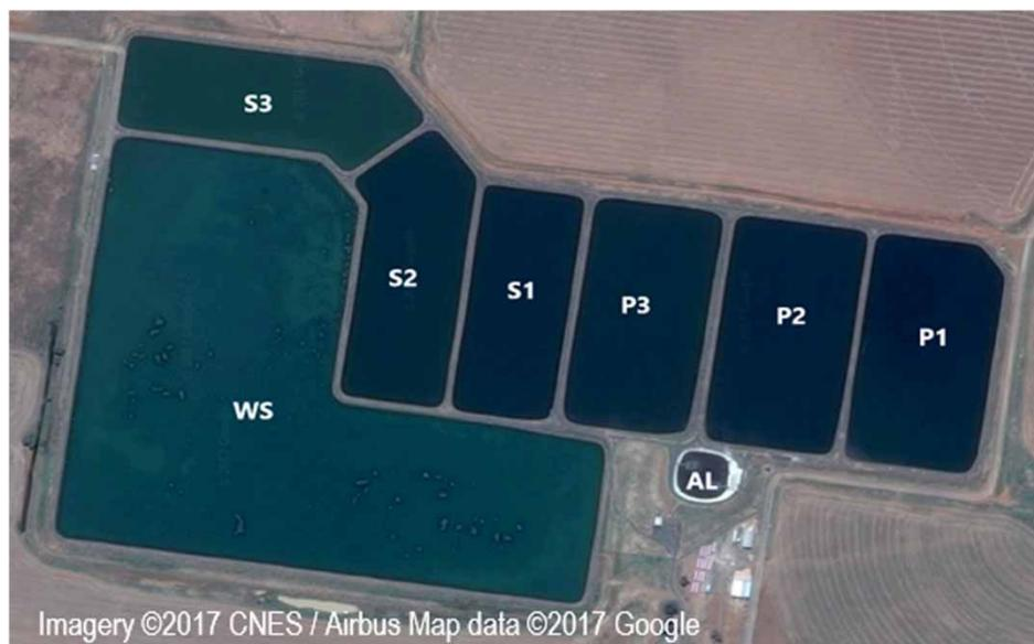
Figure 1 | Western Waters' Bacchus Marsh Recycled Water Plant. Aerobic lagoon (AL), primary lagoons (P1–P3), secondary lagoons (S1–3) and winter storage lagoon (WS) (Google Maps 2017).
