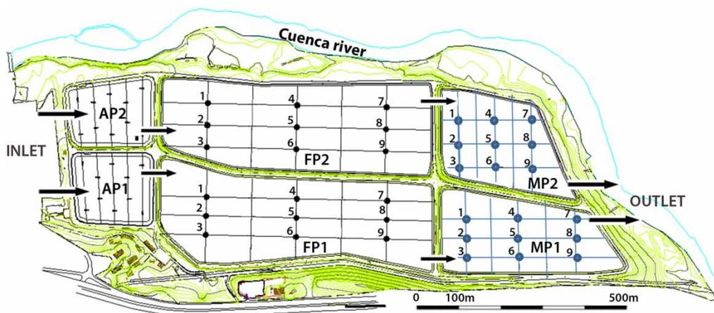
**Figure 1** | Map of Ucubamba waste stabilization pond in Cuenca, Ecuador. Two parallel lines of WSP contain aerated ponds, facultative ponds, and maturation ponds. Grids were formed within the last two ponds in order to ensure that the collected samples are representative of variations along the ponds.
