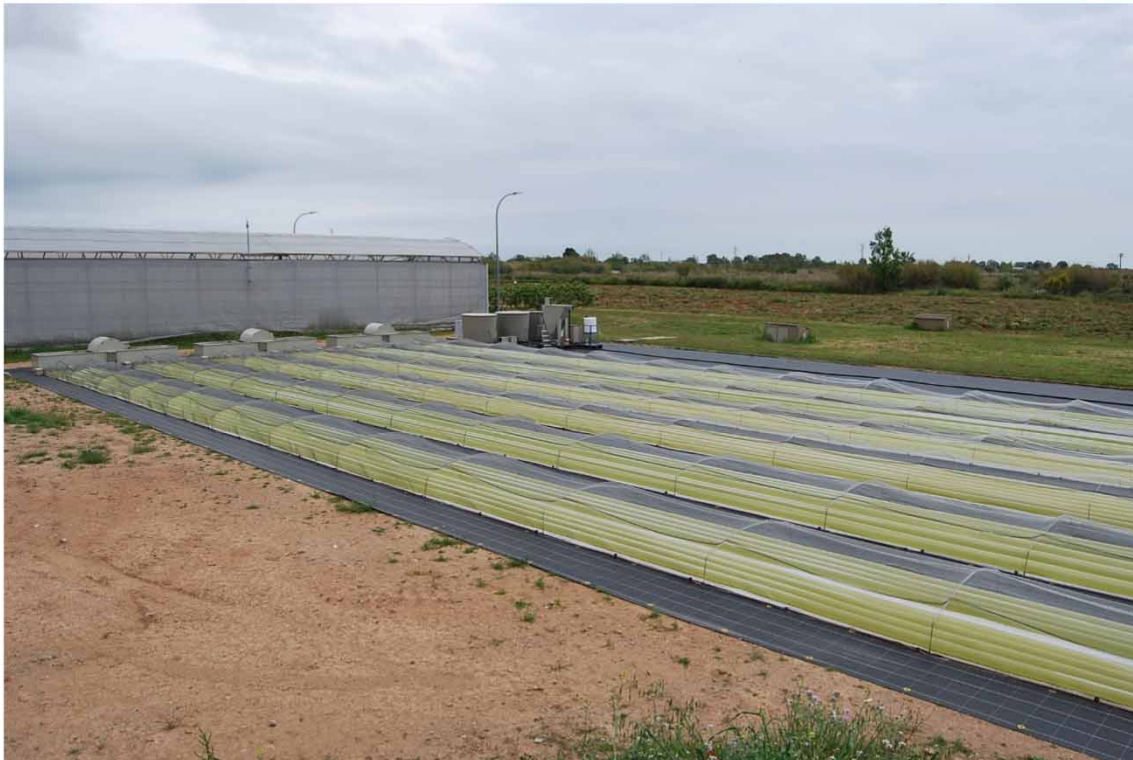
Figure 2 | Scheme of one photobioreactor and picture of the experimental plant with the three photobioreactors installed and operating.
