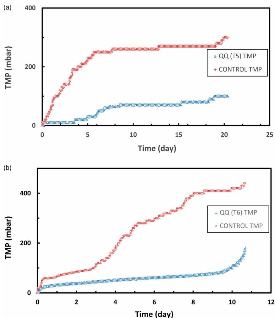
**Figure 4** | Transmembrane pressure (TMP) profiles of the control and the QQ reactors during the MBR operation with vacant beads and QQ beads with *Bacillus* sp. T5 (a) and *Delftia* sp. T6 (b).
