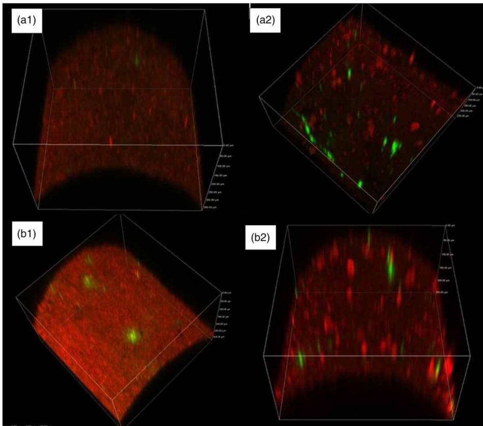
**Figure 5** | The CLSM images of biofilm formed on the membrane surfaces. (a1) Control MBR of T5 operation, (a2) QQ-MBR of T5 operation, (b1) Control MBR of T6 operation, (b2) QQ-MBR for T6 operation. Magnification:  $\times 40$ . Image size:  $501.76 \mu\text{m} \times 501.76 \mu\text{m}$ .
