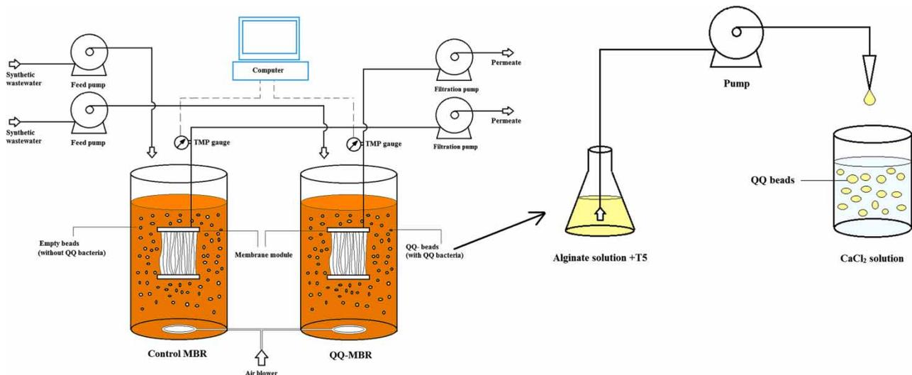
Figure 1 | Schematic diagram of laboratory-scale MBR systems and preparation of the beads.
