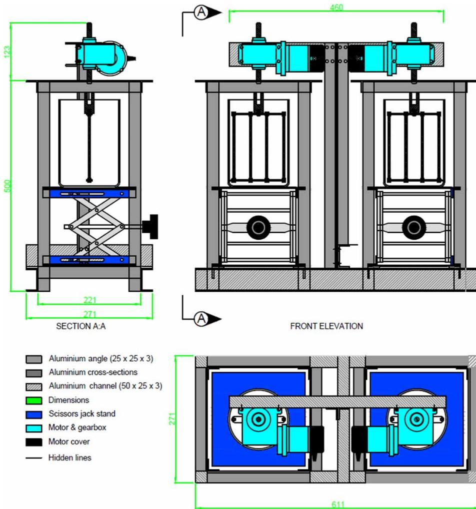
**Figure 2** | Aluminium test rig for conducting SSV tests. Included adjustable jack stands, stirring mechanism and settlement vessel. Photograph of constructed rig shown in Appendix Figure A3 (available with the online version of this paper).
