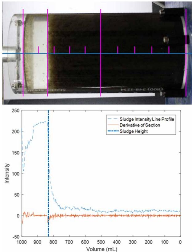
**Figure 3** | Image of partial settlement after 3 minutes. Graduated scale overlaid on vessel, with 100 mL divisions. Sludge height also marked. Plot of vertical section through mixed liquor sample and its derivative shown below it. Sludge water interface marked on both plots.
