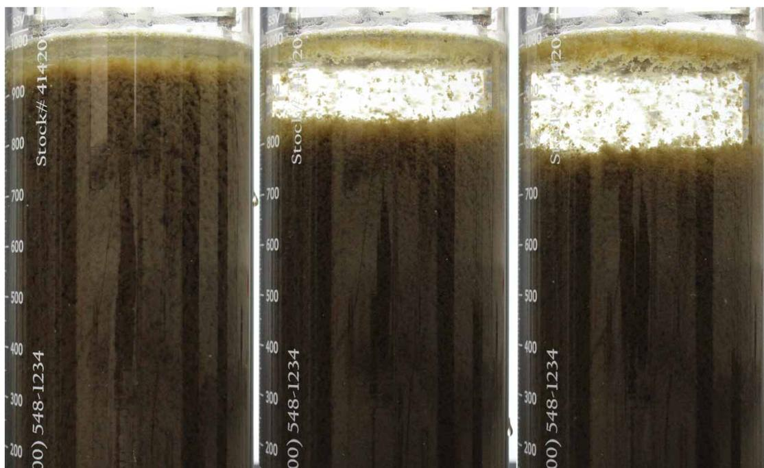
**Figure 1** | Mixed liquor sample settling in a clear vessel. A floating scum layer can be seen at the top of the vessel and a non-uniform supernatant–sludge interface as the mixed liquor sample settles.
