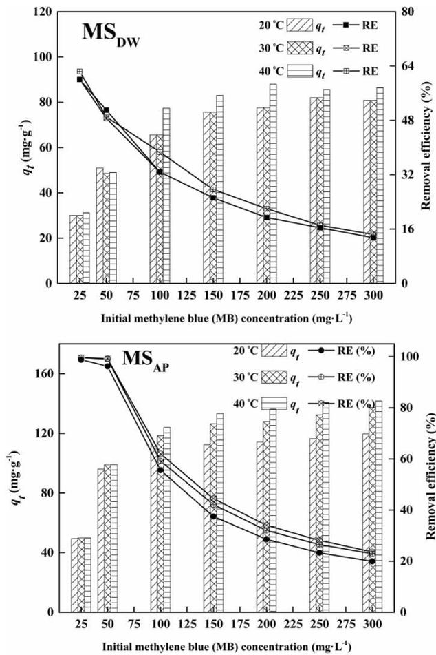
**Figure 7** | Effects of initial concentration and constant temperature on the adsorption performance.
