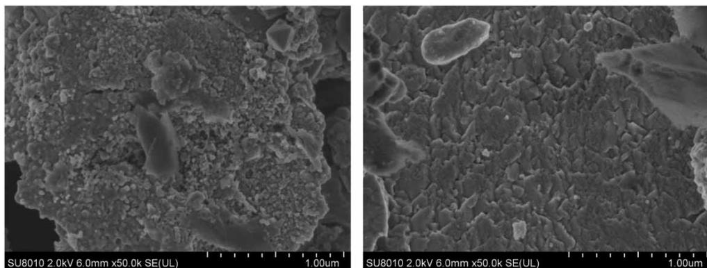
**Figure 6** | SEM images for  $MS_{AP}$  before and after MB biosorption.
