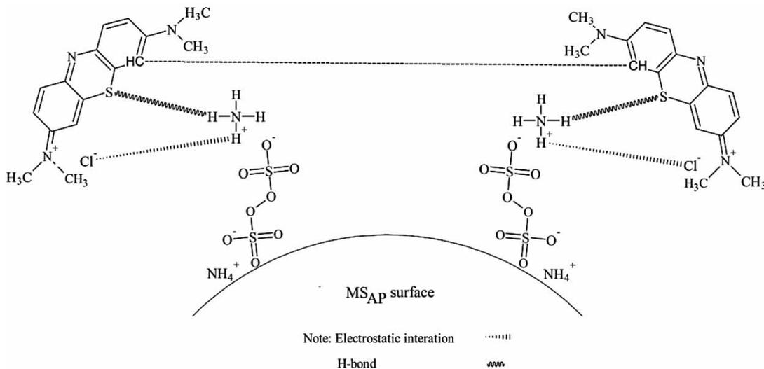
**Figure 4** | Plausible mechanism for the adsorptive removal of MB by the adsorbent chemically modified with (NH<sub>4</sub>)<sub>2</sub>S<sub>2</sub>O<sub>8</sub> (MS<sub>AP</sub>).
