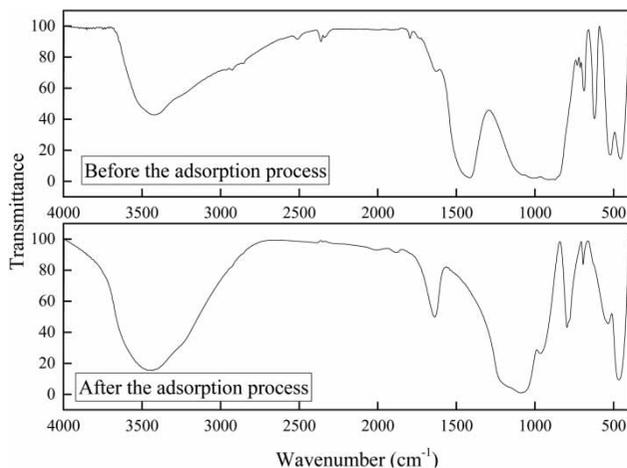
**Figure 5** | FT-IR analysis for  $MS_{AP}$  before and after MB biosorption.
