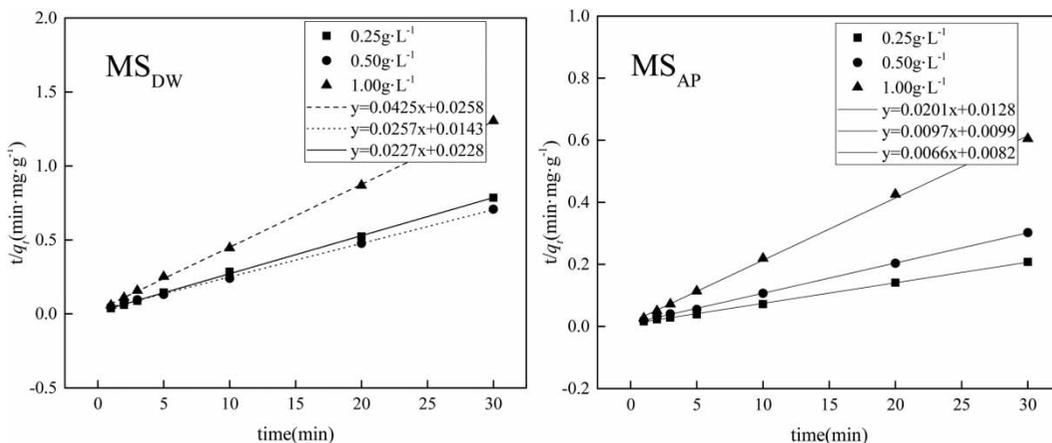
**Figure 9** | The pseudo-second-order model for the adsorption process.
