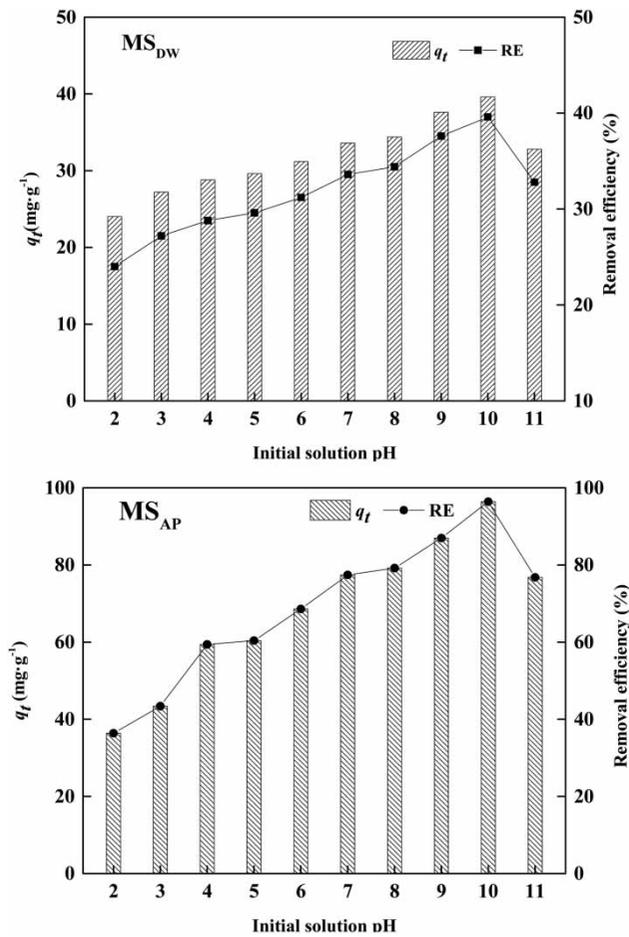
**Figure 3** | Effect of pH on the adsorption of MB onto MS<sub>DW</sub> and MS<sub>AP</sub>.
