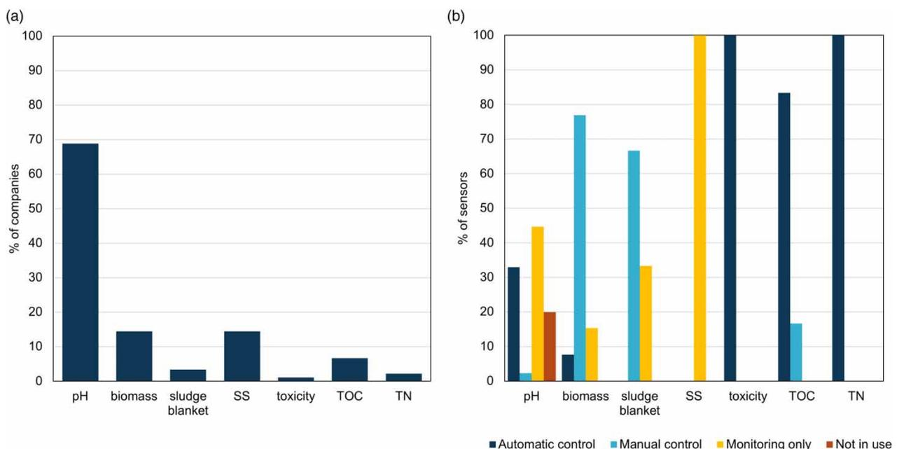
**Figure 3** | Overview of presence (a) and use (b) of online instrumentation installed on the wastewater treatment plants for pH control, sludge concentration/level control and other online instrumentation.
