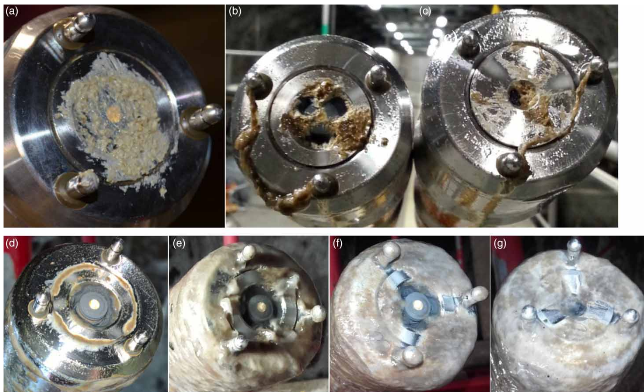
Figure 2 | (a) Artificially fouled MEC-sensor with a mixture of ball-bearing grease and pre-sedimentation grease before an experimental procedure (24 July 2015). (b) MEC- and (c) OPT-sensor after repeated air cleaning impulses (4 August 2015). Note the effect of the three air cleaning nozzles that resulted in a partly cleaned MEC-sensor in (b). Different stages of biofilm fouling on MEC-sensor (d–f) and OPT-sensor (g). Fouling time: (d) 12 days (18 October), (e) 27 days (14 November), (f) 62 days (19 December), and (g) 62 days (19 December). Note that the biofilm starts to grow in the circular gap between the sensor and the sensor body (d), and further expands over the entire sensor and rod (e, f).
