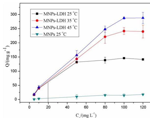
**Figure 5** | Effects of initial Orange II concentration on the adsorption capacity of Orange II on MNPs/MgAl-LDH under different temperatures. pH: 3.5,  $V$ : 10 mL,  $M$ : 2 mg, time: 50 min.
