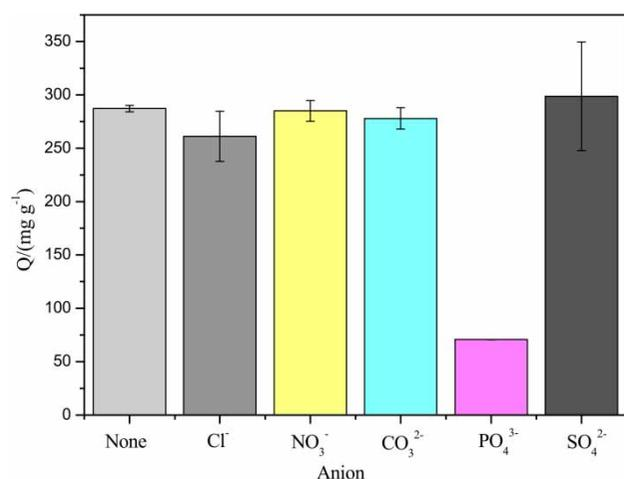
**Figure 7** | Effects of coexisting anions on the adsorption capacity of Orange II on MNPs/MgAl-LDH. pH: 3.5, V: 10 mL, M: 2 mg, T: 45 °C,  $C_{0(\text{Orange II})}$ : 100  $\mu\text{g mL}^{-1}$ ,  $C_{0(\text{coexisting anions})}$ : 100  $\mu\text{g mL}^{-1}$ .
