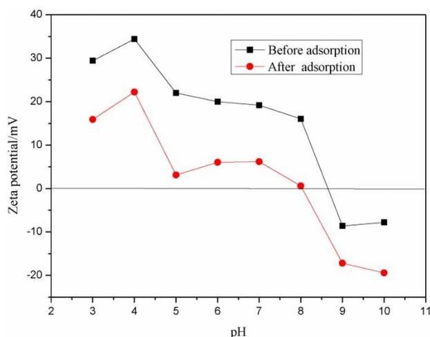
**Figure 8** | Zeta potentials of MNPs/MgAl-LDH before adsorption and after adsorption.
