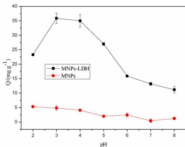
**Figure 4** | Effects of pH on the adsorption capacity of Orange II on MNPs and MNPs/MgAl-LDH.  $C_0$ :  $10 \mu\text{g mL}^{-1}$ ,  $V$ : 10 mL,  $M$ : 2 mg, time: 15 min,  $T$ :  $25^\circ\text{C}$ .
