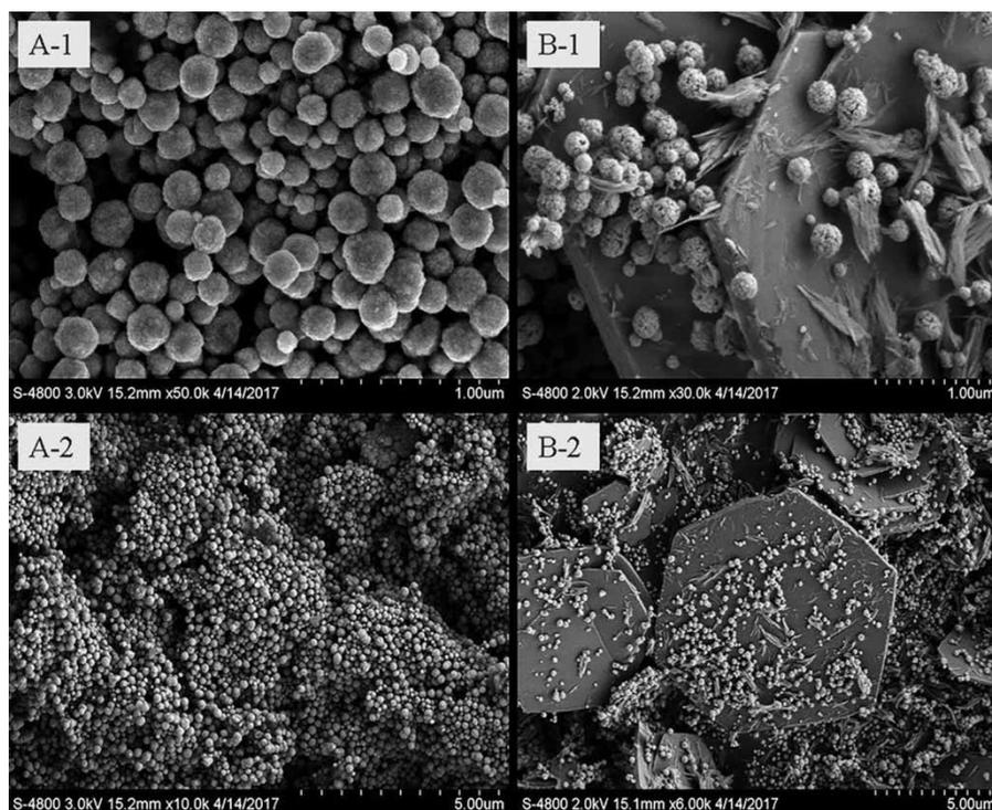
**Figure 1** | SEM images of MNPs (A-1 and A-2) MNPs/MgAl-LDH (B-1 and B-2).
