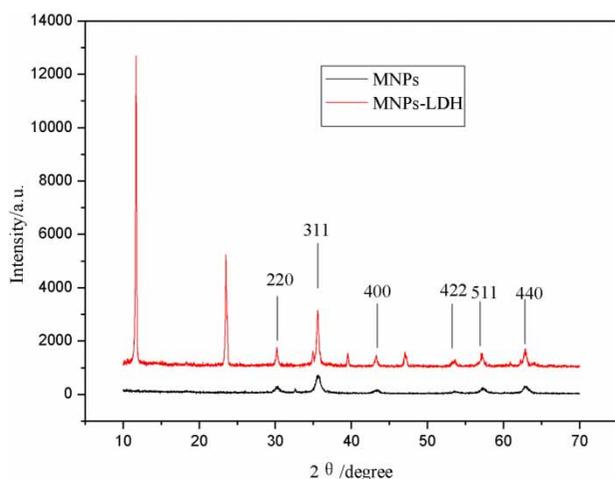
**Figure 2** | XRD pattern of MNPs and MNPs/MgAl-LDH.
