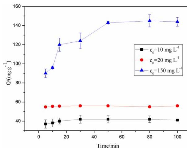
**Figure 6** | Effects of contact time on the adsorption capacity of Orange II on MNPs/MgAl-LDH under three different initial Orange II concentrations. pH: 3.5, V: 10 mL, M: 2 mg, T: 25 °C.
