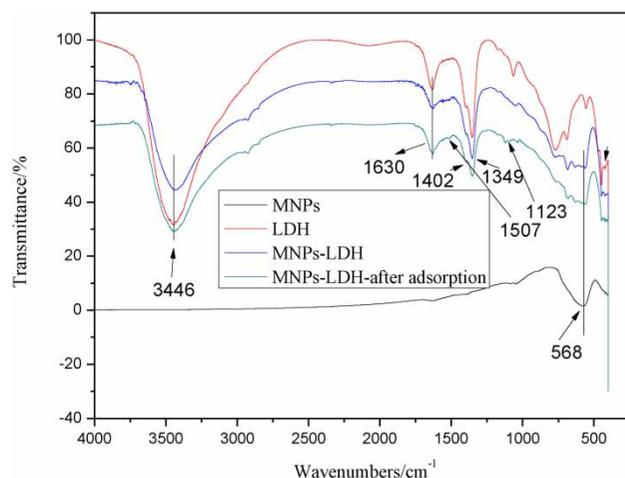
**Figure 3** | IR spectra of MNPs and MNPs/MgAl-LDH.
