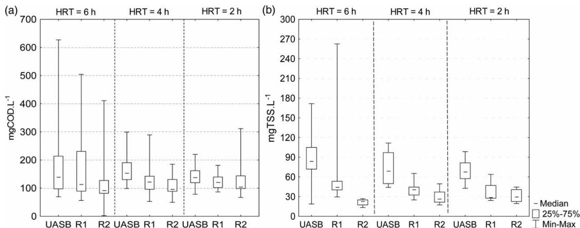
**Figure 4** | Concentrations of (a) COD and (b) TSS present in UASB and bioreactor effluents under HRTs of 6 h, 4 h and 2 h.
