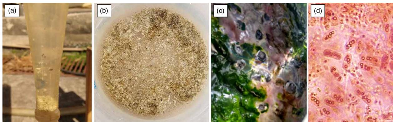
**Figure 3** | (a) Settling test of R2 - packed effluent (HRT = 6 h) after 30 minutes, with white solids at the bottom of the Imhoff cone (b) white precipitate present in the R2-packed effluent (c) picture shows the appearance of a green and purple microbial layer; (d) microscopic image of purple bacteria in R2-packed biomass (HRT = 4 h), emphasizing intracellular sulfur.
