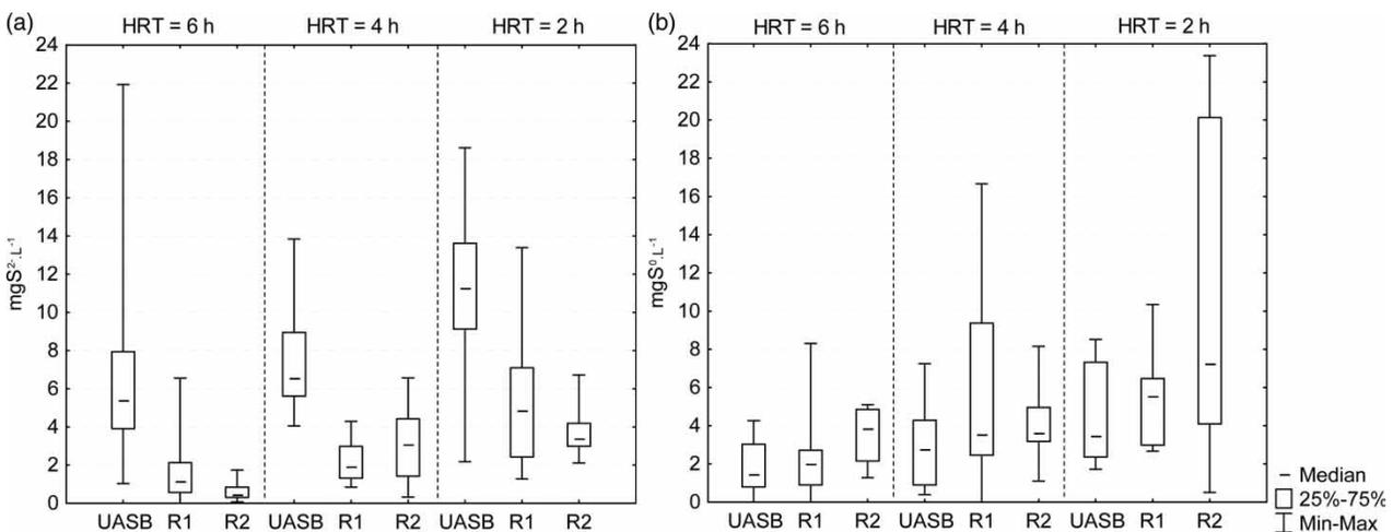
**Figure 2** | (a) Dissolved sulfide and (b) elemental sulfur concentrations in the effluent of the UASB reactor and phototrophic bioreactors. R1: control reactor and R2: packed reactor (polypropylene rings).
