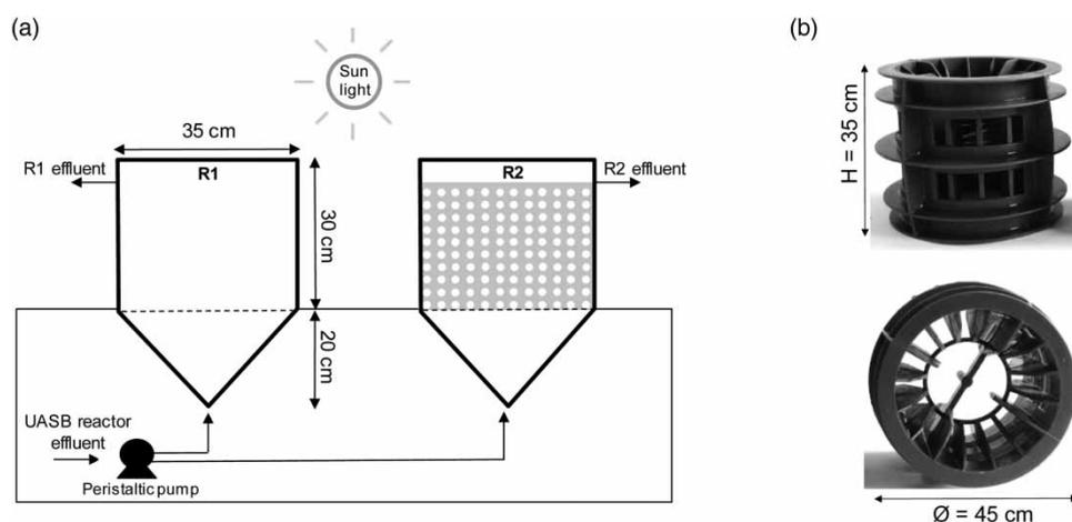
**Figure 1** | Schematic representation and dimensions of (a) bioreactors and (b) packing material adopted in this work.
