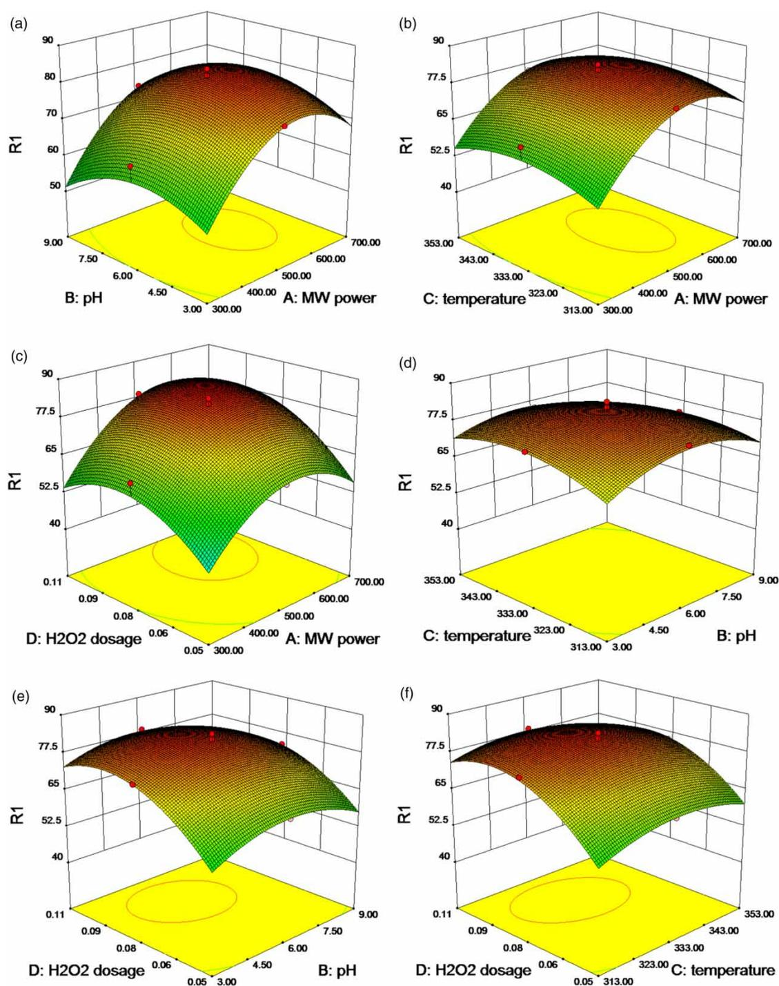
**Figure 4** | Response surface showing effect of interaction of (a) microwave power and pH, (b) microwave power and temperature, (c) microwave power and H<sub>2</sub>O<sub>2</sub> dosage, (d) temperature and pH, (e) pH and H<sub>2</sub>O<sub>2</sub> dosage, and (f) temperature and H<sub>2</sub>O<sub>2</sub> dosage on mineralization efficiency of quinoline.
