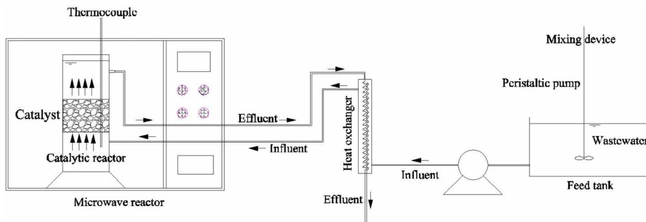
**Figure 1** | Experimental device for microwave assisted catalytic wet hydrogen peroxide oxidation.
