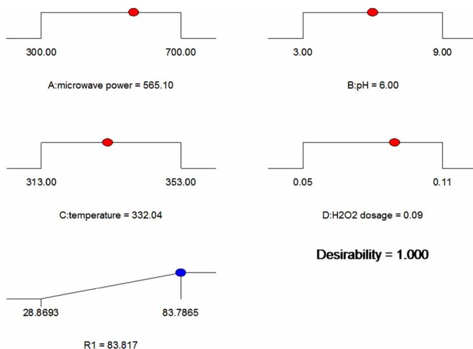
**Figure 5** | Optimized process condition for quinoline mineralization efficiency.
