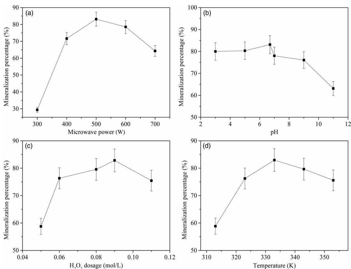
**Figure 2** | The independent effect of parameters on quinoline mineralization: (a) microwave power, (b) initial pH value, (c) H<sub>2</sub>O<sub>2</sub> dosage, and (d) temperature.
