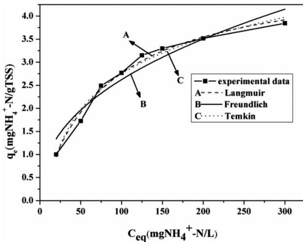
**Figure 3** | Adsorption isotherms and fitted curves for ammonium adsorption.
