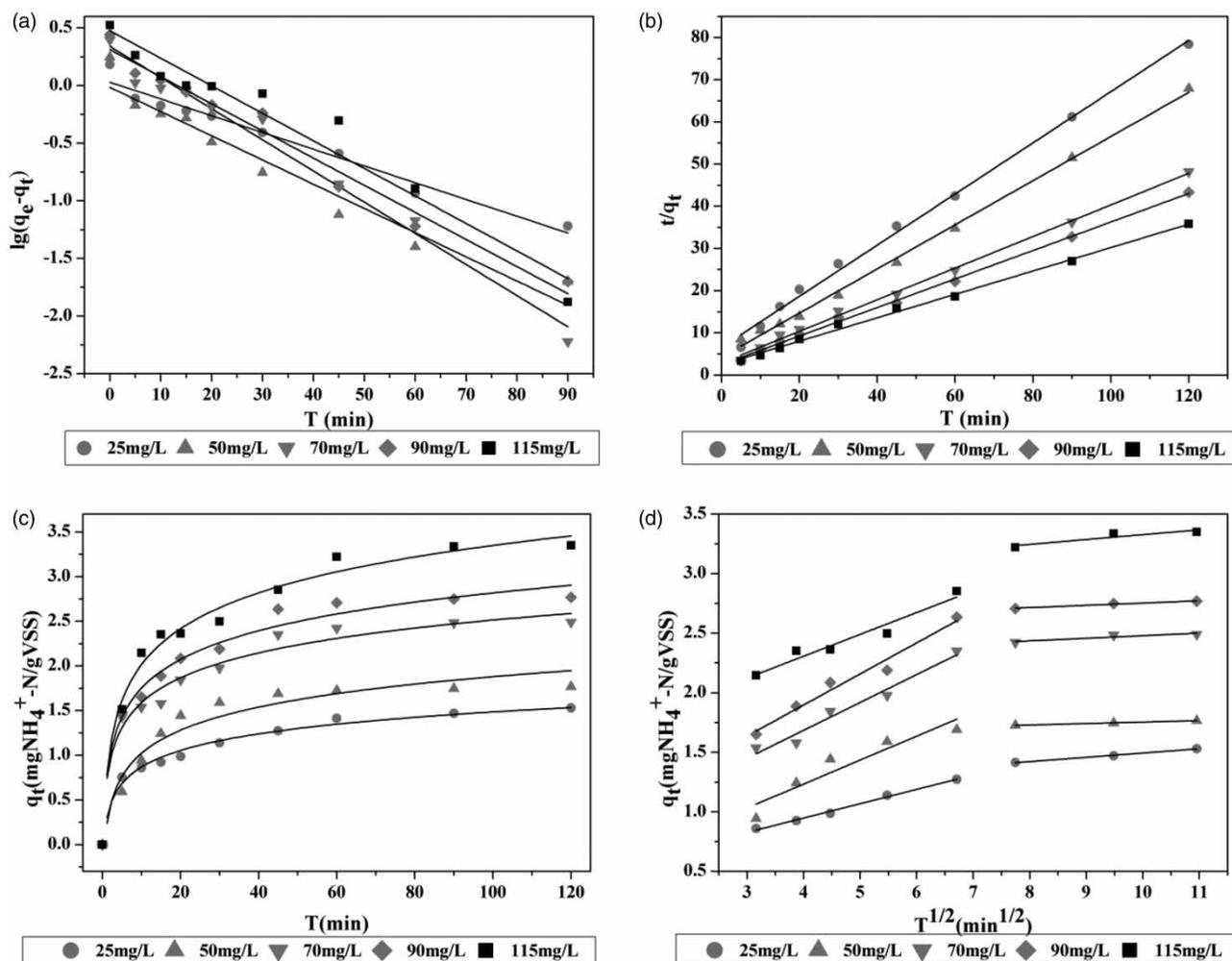
**Figure 2** Kinetic models of ammonium adsorption: (a) pseudo-first-order, (b) pseudo-second-order, (c) Elovich model and (d) intra-particle diffusion under different initial ammonium concentration.
