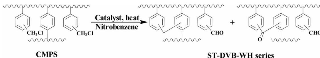
Figure 1 | Schematic procedure for synthesis of ST-DVB-WH series resins.
