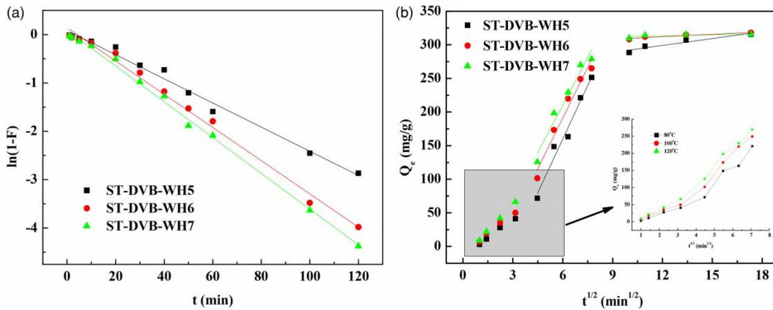
**Figure 5** | The fitting of the film diffusion model (a) and intra-particle diffusion model (b) of ST-DVB-WH5, ST-DVB-WH6 and ST-DVB-WH7.
