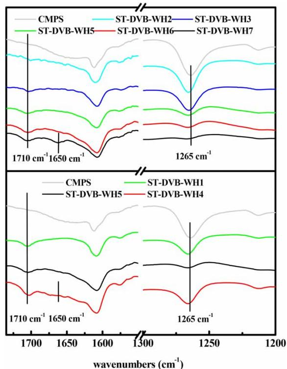
Figure 2 | IR spectra of ST-DVB-WH series resins.
