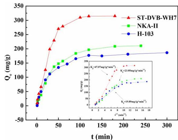
**Figure 6** | The result of the adsorption kinetics and intra-particle diffusion model of ST-DVB-WH7, NKA-II and H-103.
