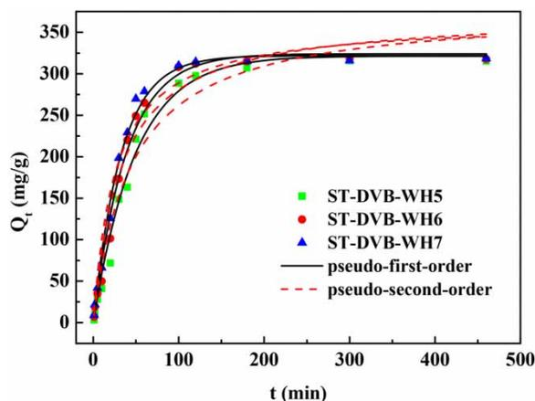
Figure 4 | The adsorption kinetics of ST-DVB-WH5, ST-DVB-WH6 and ST-DVB-WH7.
