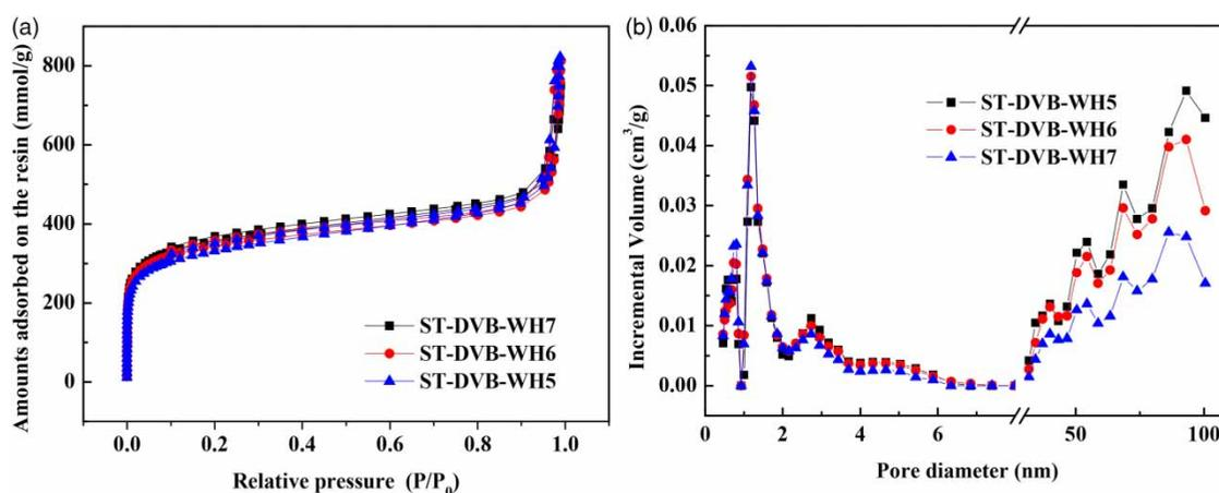
**Figure 3** | N<sub>2</sub> adsorption-desorption isotherms (a) and pore size distribution vs incremental volume (b) of ST-DVB-WH5, ST-DVB-WH6 and ST-DVB-WH7.
