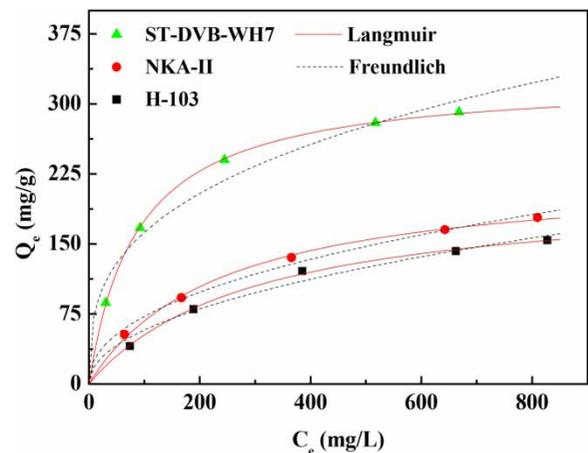
**Figure 7** | The result of the adsorption isotherm of ST-DVB-WH7, NKA-II and H-103.
