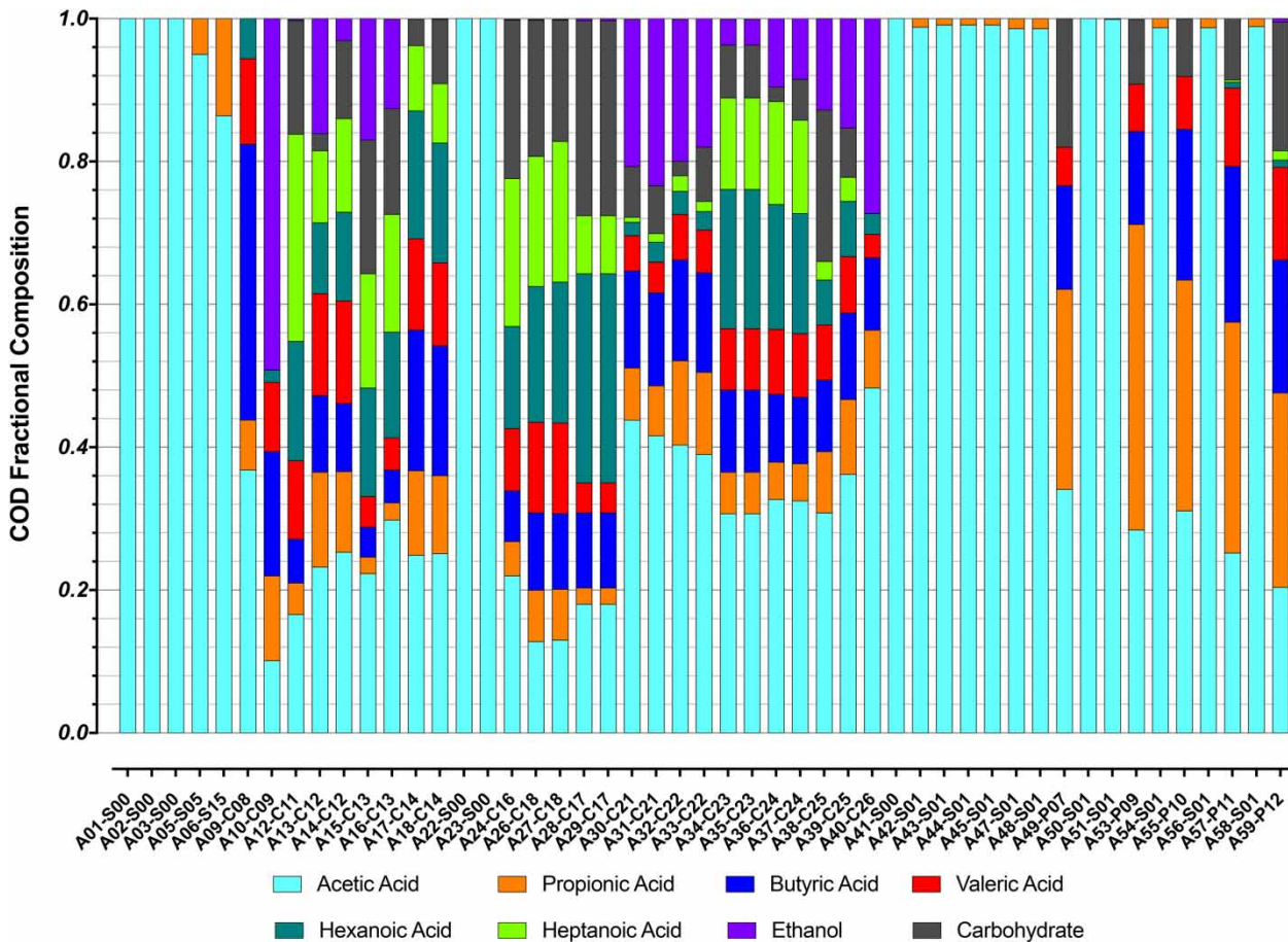
Figure 2 | Relative COD composition of the range of feedstocks used to produce batches (A01 to A59) of PHA-rich biomass over the 10 months of pilot plant operations. Non-VFA COD is expressed as carbohydrate. The feedstocks were batches of synthetic VFA mixtures (Sxx), fermented candy factory process effluent (Cxx), and fermented Waterschap De Dommel primary sludge centrate (Pxx).
